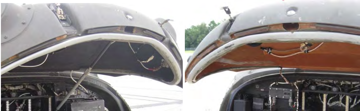
Figure 16. UH-60 NDS after 90 days in the field, baseline (left) and alternate (right).
