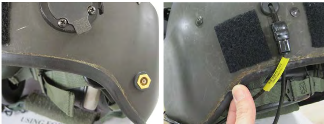
Figure 18. Aviation helmet after 180 days in the field, baseline (left) and alternate (right).
