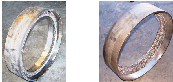
Figure 13. As-deposited PTA demonstration cases
