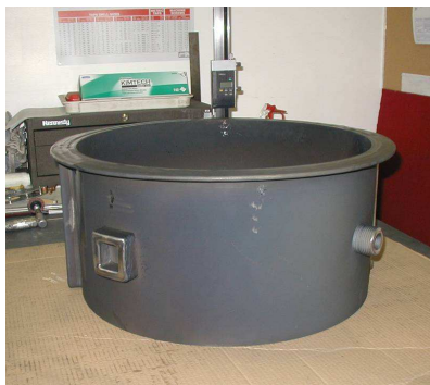
Figure 10. As-deposited eBAM demonstration case
