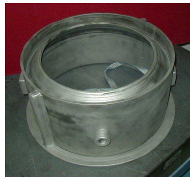
Figure 10. As-deposited eBAM demonstration case
