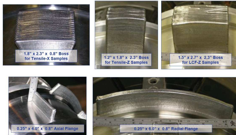
Figure 7. GE Task 4 LAM deposits on Alloy 718 Ring
