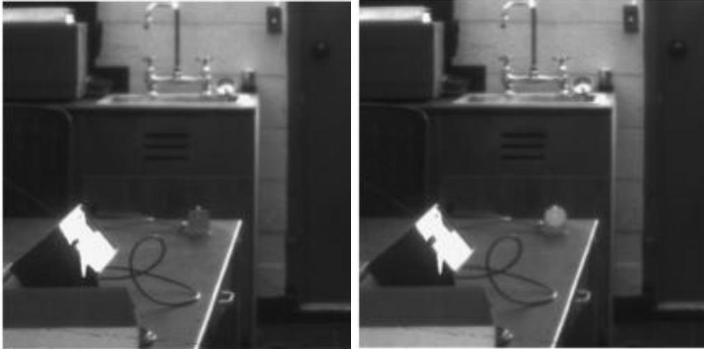
Figure 11. 270 nm LED in “off” (left) and “on” (right) conditions as viewed by intensified PentaMAX camera sensitive to both ultraviolet and visible light.
