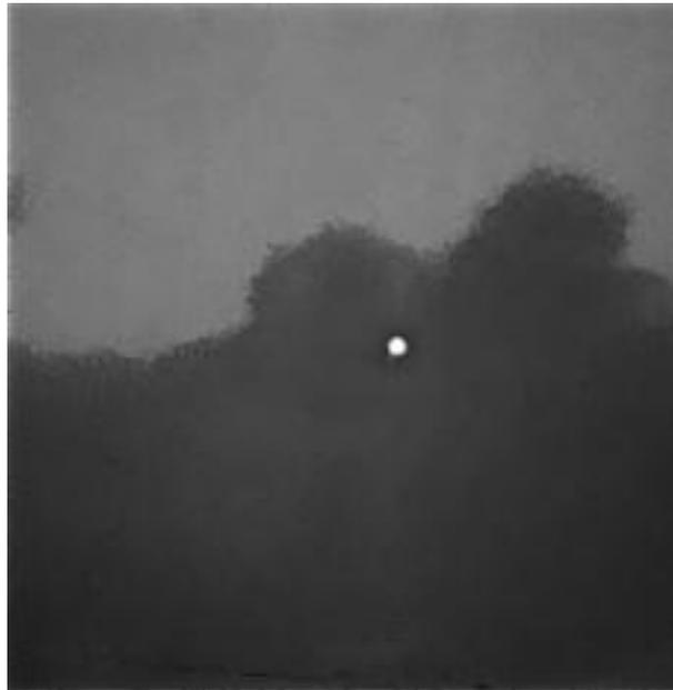
Figure 37. Daytime image of four 270 nm HS LEDs each with 70 mA driving current viewed from 300 m through 270N and 270B solar blind filters with 150 ms exposure time.
