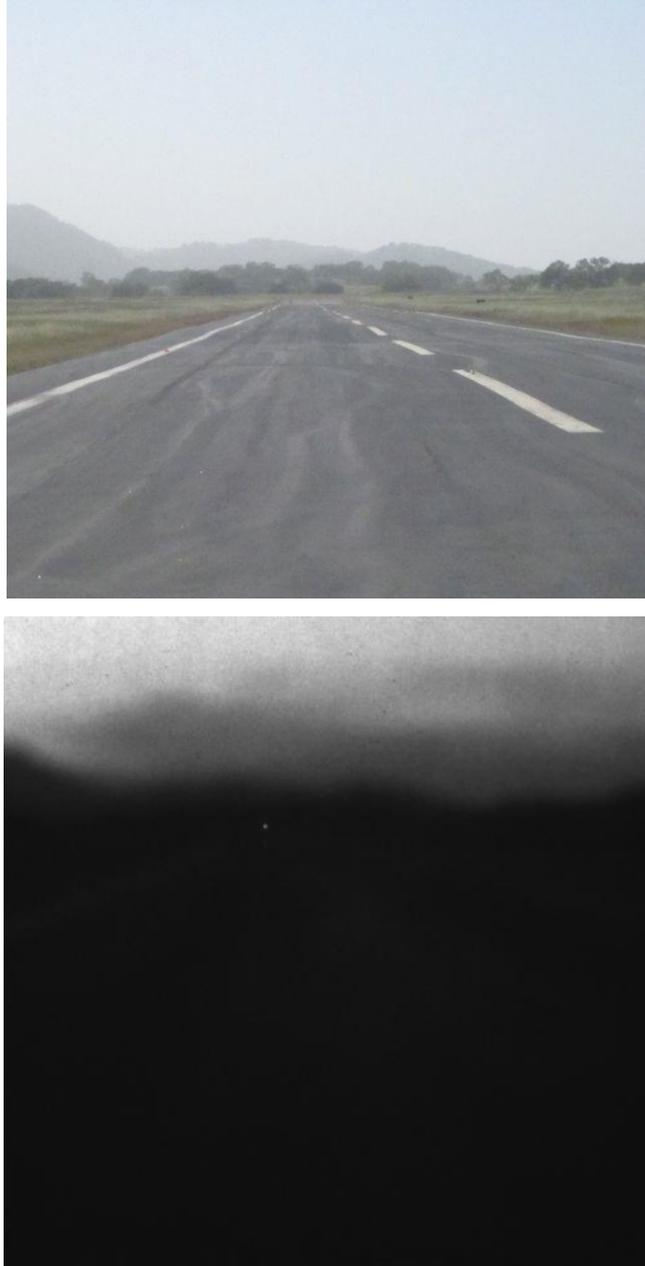
Figure 47. Daytime images of prototype device viewed from 980 m by visible camera (Top) and intensified PentaMAX camera with 270N and 270B solar blind filters and 30 ms exposure time (bottom). In the second image, the prototype is the white dot shown just below the horizon.
