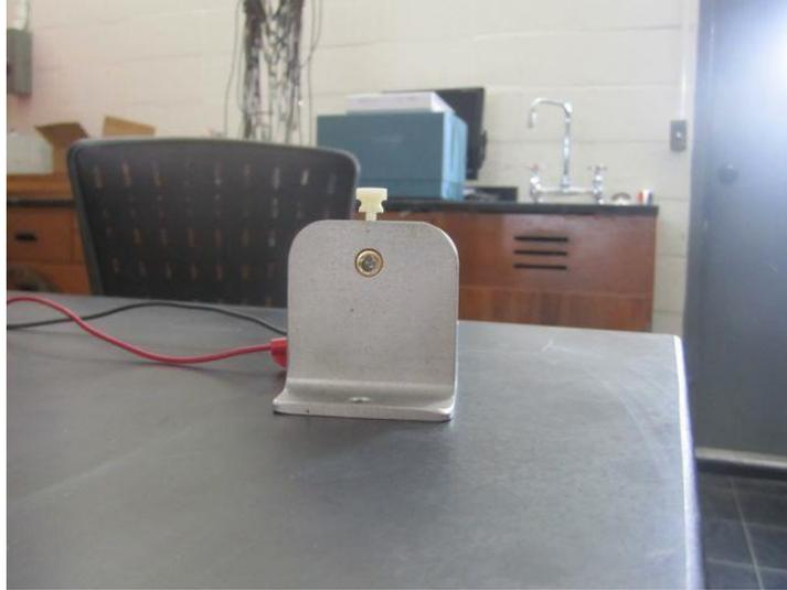
Figure 9. Close-up view of mount used to hold LED.
