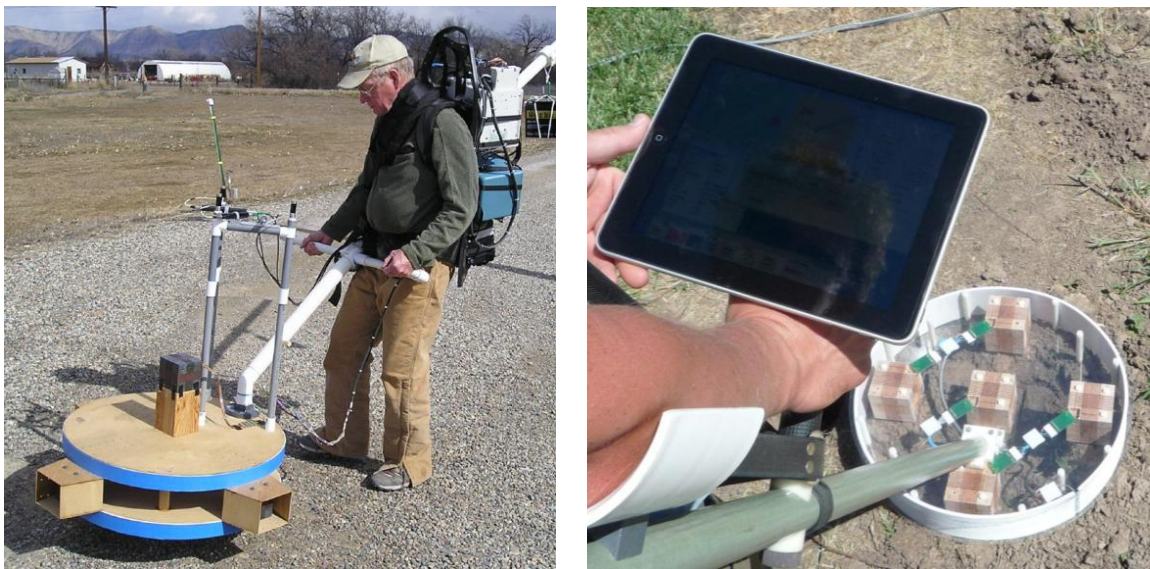
Figure 4: MPV prototype development. Right: original sensor (head weights 23 lbs). Left: second generation sensor with touch-screen control display (head weights 12 lbs).
