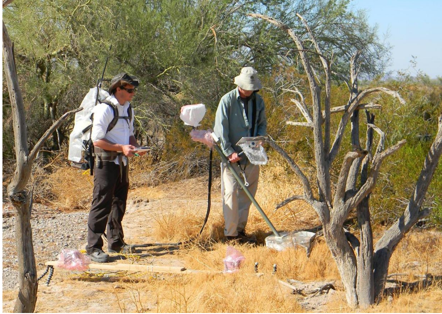
Figure 29: MPV2 field data collection. Surveying generally requires two persons. The main operator carries the sensor with one arm and interacts with the control interface display with his spare hand. The second operator carries the DAQ backpack, takes field notes and monitors the survey for any potential difficulty.
