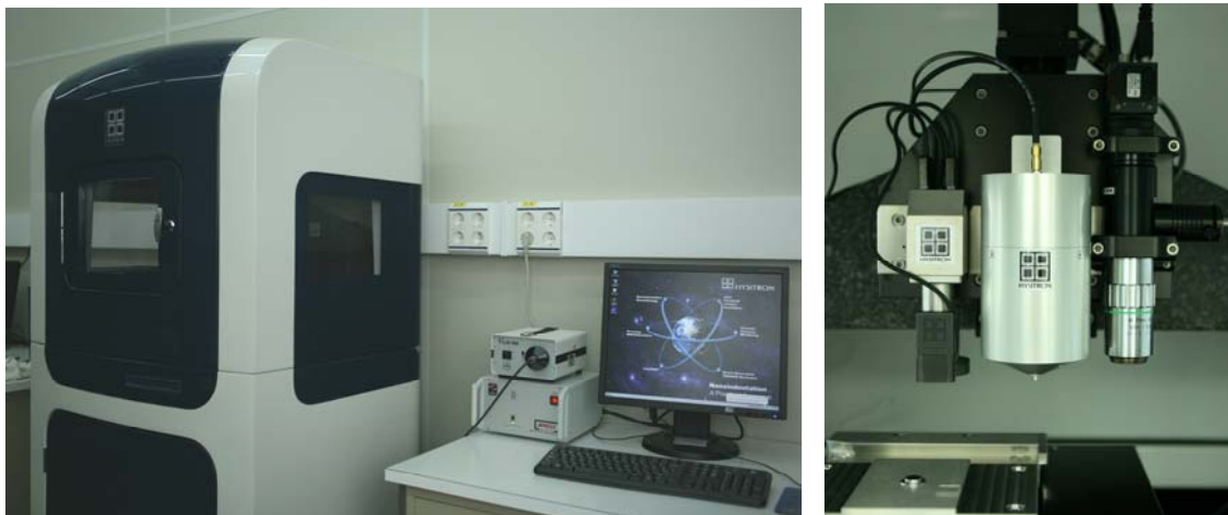
Figure 2: Nano-Indenter TI-950 from Hysitron. General view of the installation and detail of the measuring heads, with (from left to right) the low load transducer, the high load transducer and the optical microscope.
