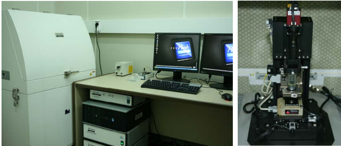
Figure 2: Nano-Indenter TI-950 from Hysitron. General view of the installation and detail of the measuring heads, with (from left to right) the low load transducer, the high load transducer and the optical microscope.
