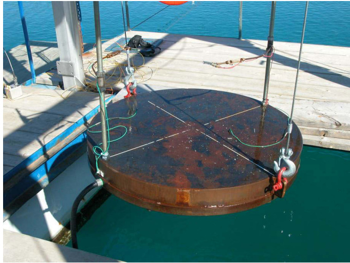
Figure 3: Target plate used for the rigid plate experiments conducted at DRDC Suffield
