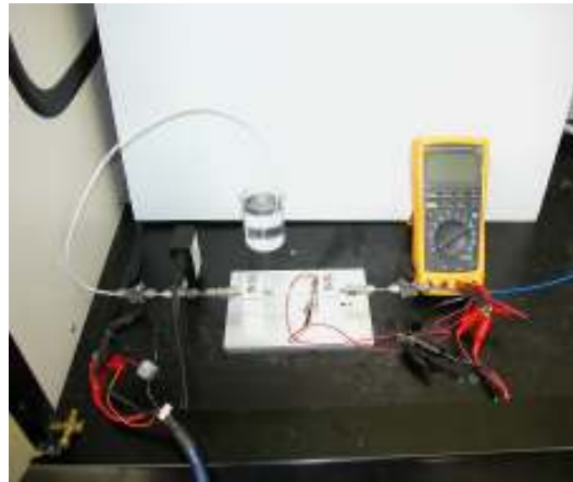
Figure 9. Photo of test fixture comprising the fiber holder, cables leading to a MACOR 4300 programmable electronic load, tubing leading to gas (nitrogen and hydrogen) handling equipment, a suite of sensors including pressure, temperature, and humidity. The beaker of water in the upper left enables visual detection of flow during flushing operations, and prevents air from diffusing back into the fiber.
