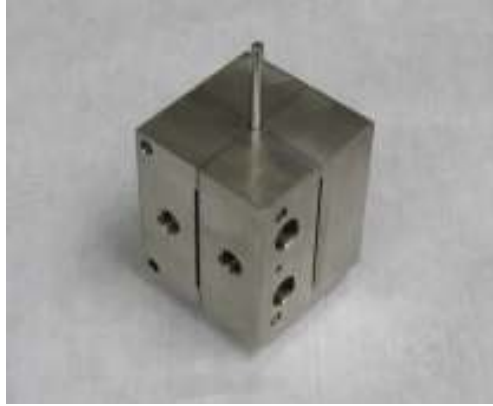
Figure 6. Photo of die used for pressing LiAlH 4 fuel pellets
