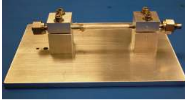
Figure 8. Photo of fiber fuel cell in the fiber holder
