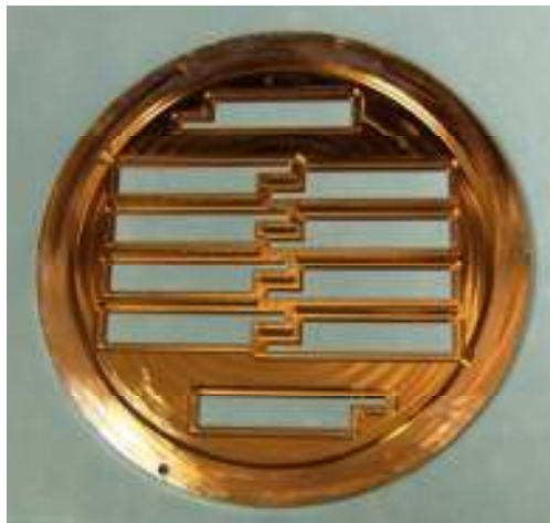
Figure 5. Photo of shadow mask used for patterning metal on the fiber electrodes
