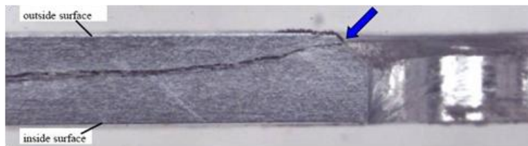
Figure 25. Cracking on A/C 68-0222 (Including Cross-Section)
