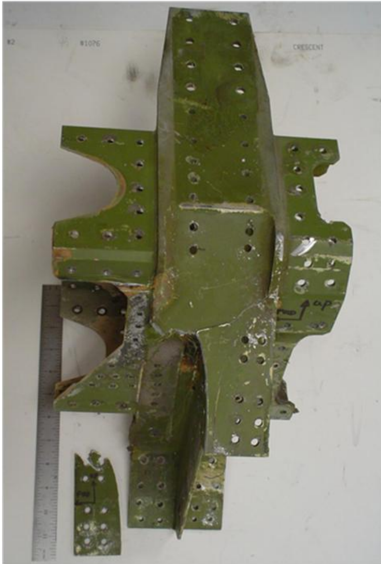
Figure 17. Damaged Contour Box Beam Fitting
