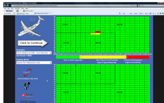
Figure 66. CBM System Mock Up – SHM System Implemented
