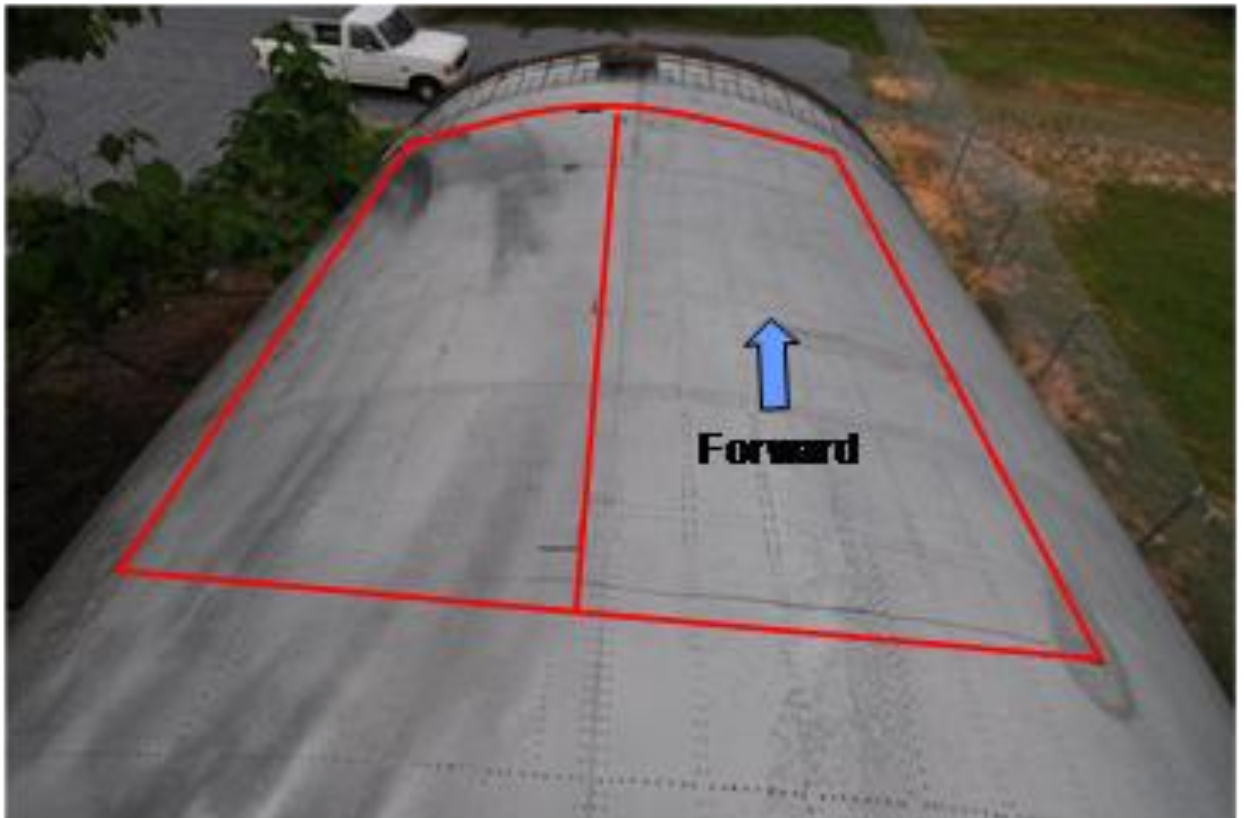
Figure 28. Top View of X997 with section to be removed in red
