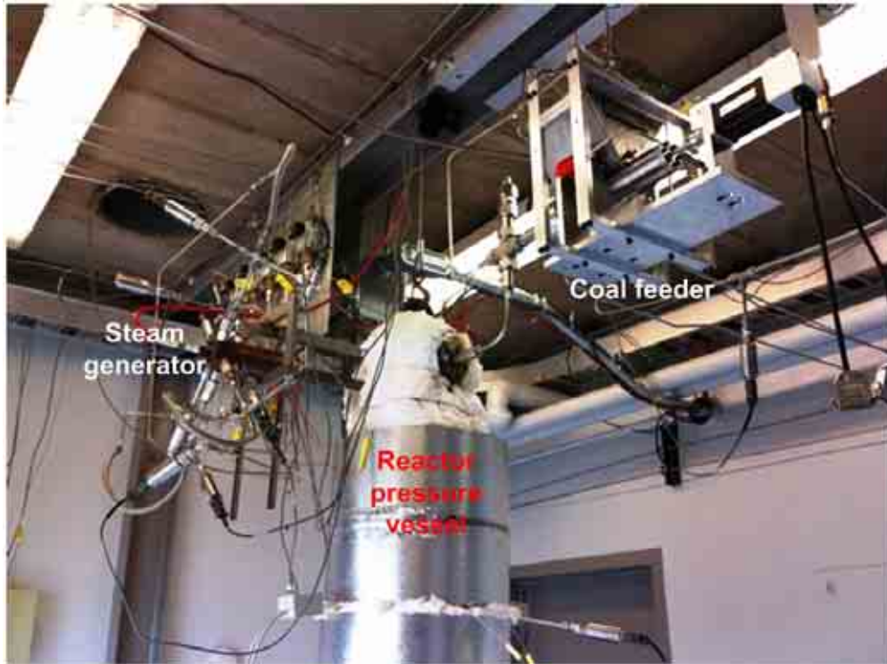
Figure 2.2: Gasifier reactor, hydrogen-oxygen steam generator and coal/biomass feeder in the experimental test cell.
