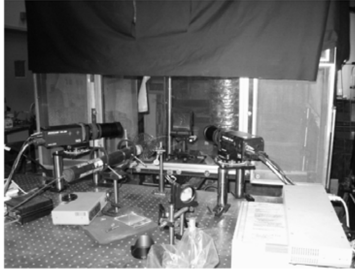
Figure 3.1: Experimental SPIV system. The counter-flow burner is located inside the enclosure to avoid spreading of seed particles.
