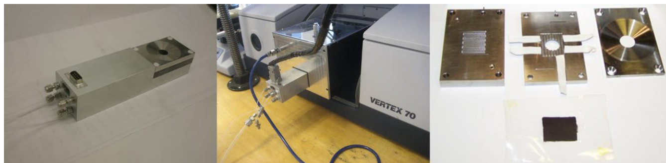
Figure 1: IR-XAS cell. Top: Red path, reflectance IR or fluorescence XAS; yellow path; transmission XAS. Bottom left: Assembled spectroscopy cell with DE9 connector for electrodes, heater cartridge and thermister. Bottom center: Cell installed in Pike diffuse reflectance accessory in a Bruker (Billerica, MA) Vertex 70 FTIR Spectrometer. Bottom right:
