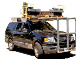
Figure 1: The ARL UWB SIRE radar system integrated on the Ford Expedition.
