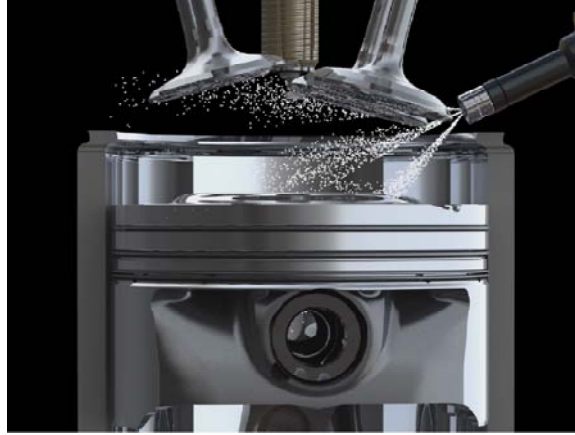
Figure 43. Schematic of the 3.5-L V6 EcoBoost combustion system with multihole GDI injector (77).
