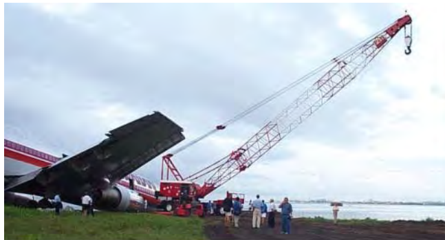
Figure 3. Crane Positioning for Lift
