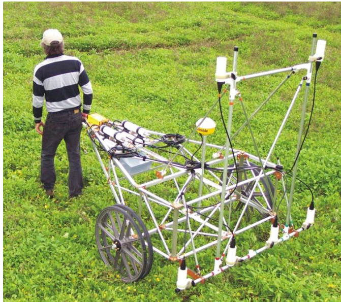
Figure 3. Array of current generation sensors for land surveying application. Smaller sensor systems would greatly reduce the size and complexity of such platforms.
