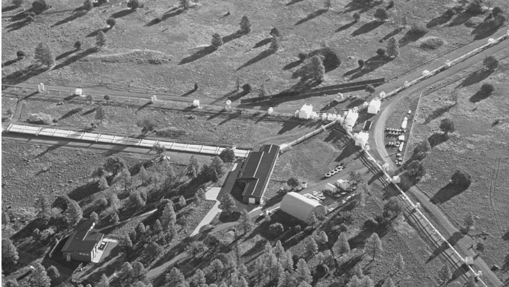
Figure 1. The Navy Prototype Optical Interferometer (NPOI). The north arm is the one extending to the left of the center of the array. Feed pipes lead from the array center to the optics laboratory, which houses the continuously-adjustable “fast delay lines.” Extending to the north of the optics laboratory is the array of “long delay lines” that will provide additional delay when the longest baselines are commissioned. Close to the center of the array are the four enclosures for the astrometric array elements, which are fixed in position. The east and center astrometric array elements were used for these observations, along with one of the moveable imaging array elements, E6, visible just above and to the right of the east astrometric enclosure. Photo courtesy of Michael Collier.
