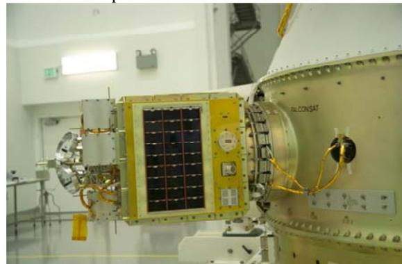
Figure 5. FalconSAT-3 mounted on ESPA Ring
