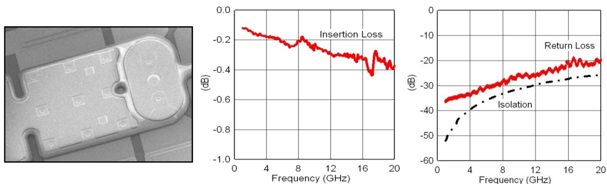
Figure 2: XCOM RF MEMS switching element and S-parameters of relay die.
