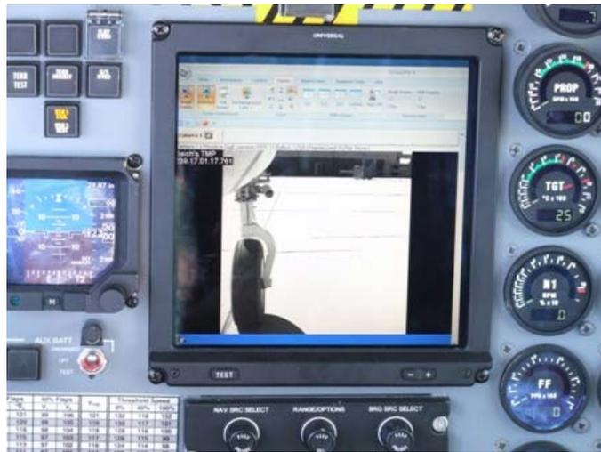
Figure 4.13: Pilot display showing real-time camera view. This modification allowed the pilots to accurately fly the aircraft to collect the required visual data.
