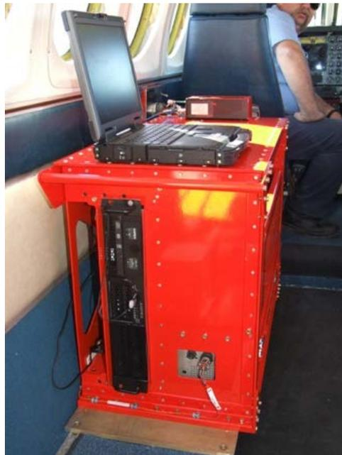
Figure 4.12: Installed equipment rack with tower computer beneath and laptop velcroed on top. The laptop controlled the rest of the hardware through a remote desktop connection.
