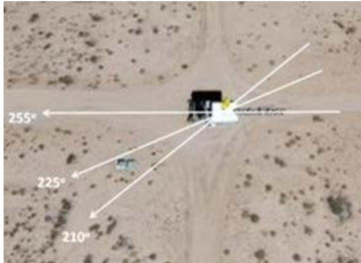
Figure 4.19: Run-in headings against Cowbell Tower. The magnetic headings shown correspond to 0°, 30°, and 45° from a heading chosen as perpendicular to one side of the tower cab.
