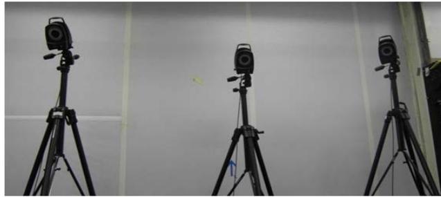
(c) Three of the 10 cameras arranged in a circle around the test area in the Vicon<sup>®</sup> lab.
