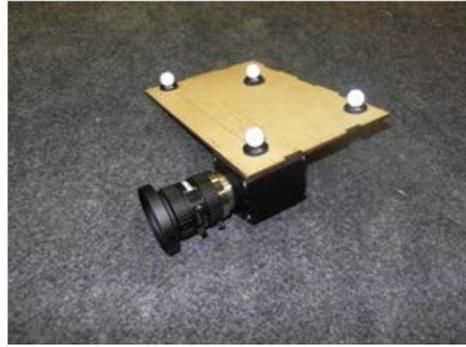
(b) Board with four tracking spheres glued to test camera.
