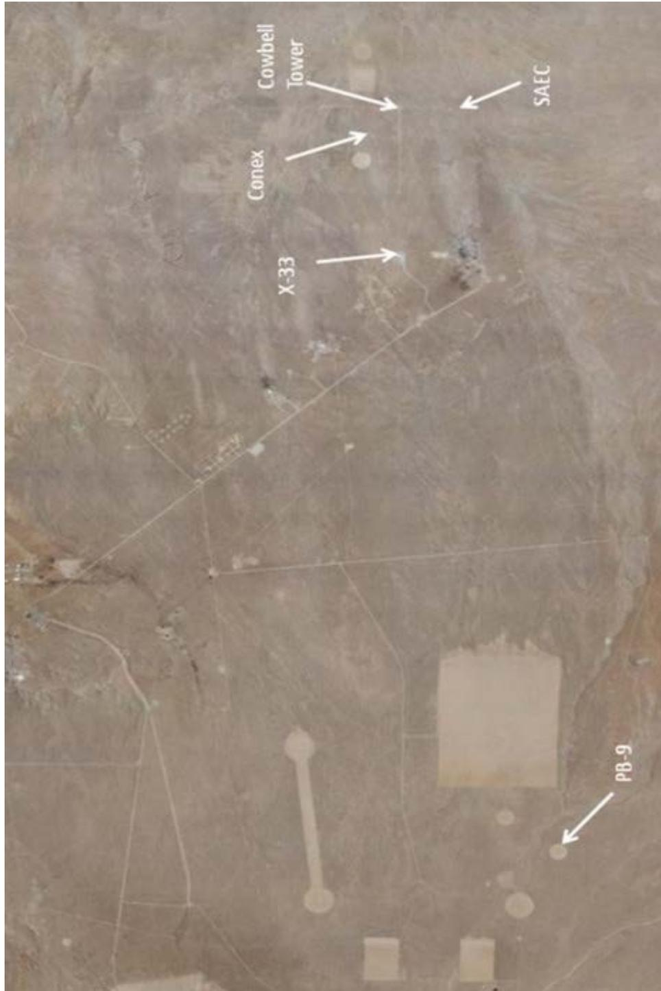
Figure 4.16: Location of targets on PIRA. The top of the photograph is north; the Edwards AFB runways are to the left of the image (not shown). The distance from Cowbell Tower to PB-9 is 9.2 statute miles.
