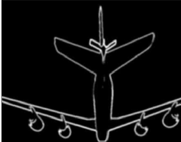
Figure 2.10: Gradient image of KC-135 from Weaver’s research [37]. This method worked well for a lone object against a blank background (sky).
