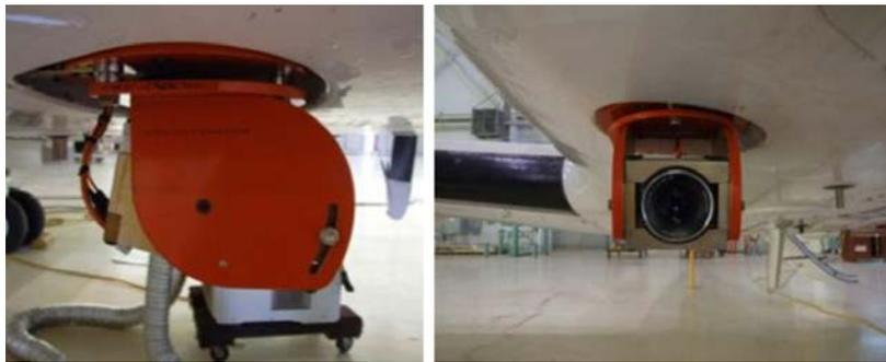
(b) Camera mounted through driftmeter port under copilot on C-12C.
