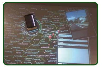
Data from the Tactical Ground Reporting (TIGR) system is seamlessly transferred between a smartphone and multitouch table using COMET.
