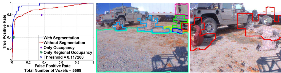
(d) Two manikins introduced into the scene were detected perfectly. The second was pinned underneath the vehicle, making accurate detection of this manikin especially difficult.
