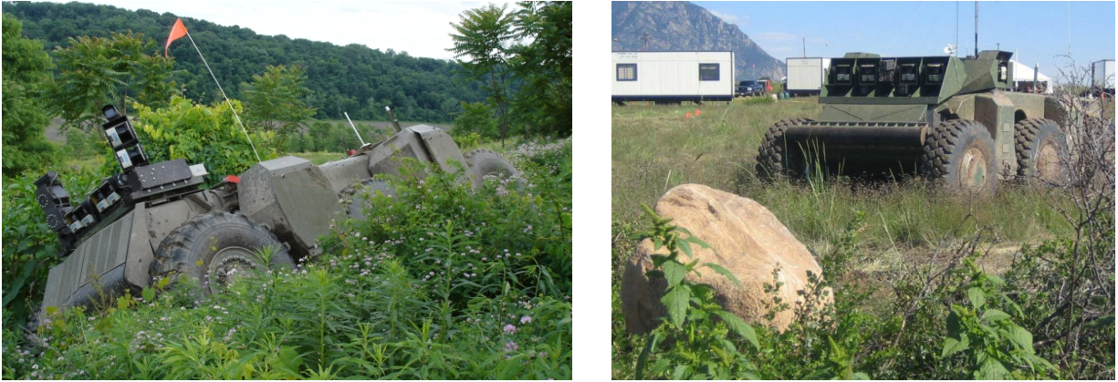
Figure 3.3: Spinner (left) and Crusher (right) robots used for experimentation throughout earlier thesis work. The natural terrain shown here is representative of the domains they operate within.
