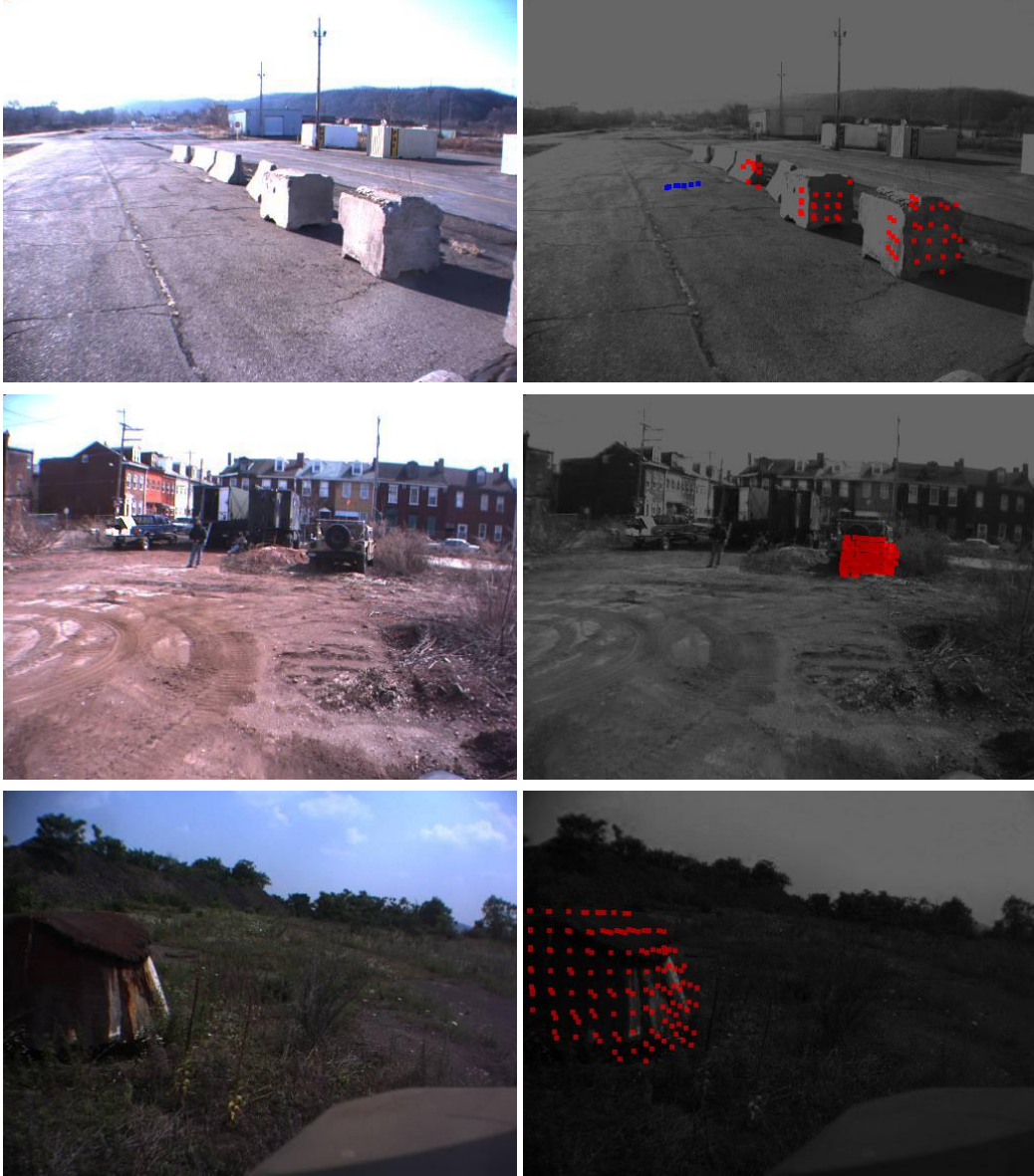
Figure 5.9: Sample labeled examples in the 'other man-made' class used for validation of dimensionality reduction effectiveness. This category excluded instances of barrels which were used as a separate known class.
