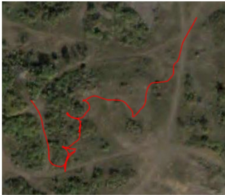
Figure 1.2: UGVs navigating with a limited perception range will often execute highly suboptimal paths. The path above was executed by a large UGV whose goal was to navigate to the goal at the left portion of the environment using an onboard perception system with a range of approximately 15 meters. Due to its limited visibility range, the UGV lost significant time navigating through the heavy vegetation while taking heavy risks in the process that necessitated a human intervention at one point.
