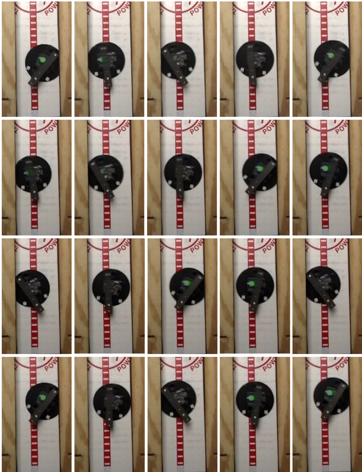
Figure 3.24: DSAC Period-1 experiment - \omega = 17.3 \frac{\text{rad}}{\text{s}} , A = 0.28 \text{rad} and \gamma = 0.869 – image sequence approximately 10ms apart.
