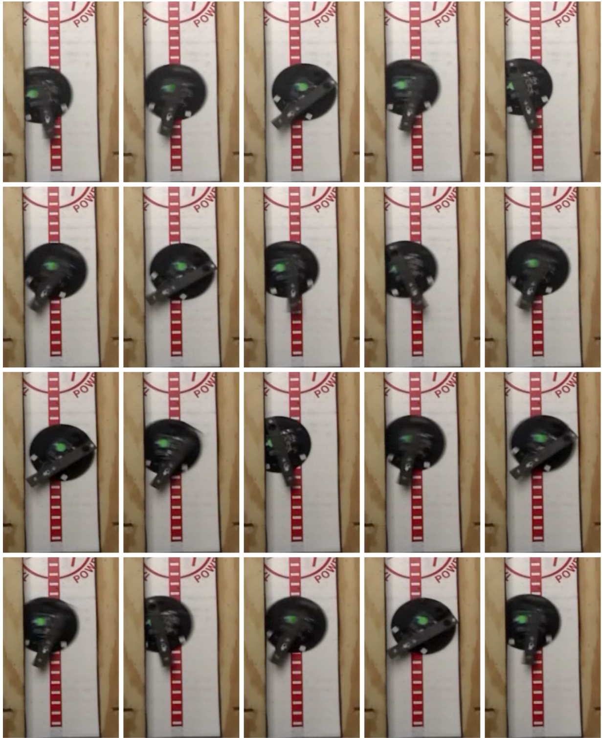
Figure 3.28: DSAC Period-2 experiment: \omega = 16.5 \frac{\text{rad}}{\text{s}} , A = 0.27 \text{rad} and \gamma = 0.769 – image sequence approximately 15ms apart.
