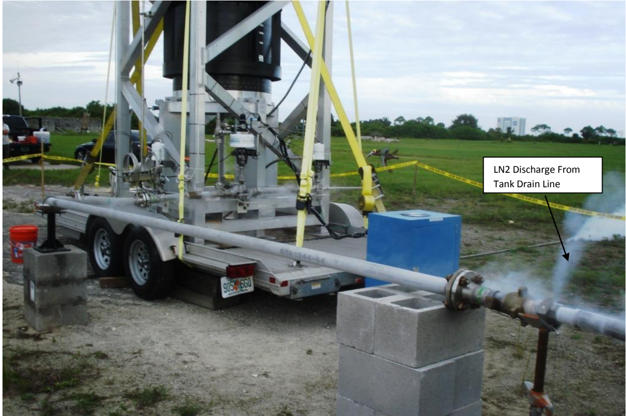
Figure C-7 Start Of Chill-down, Run 1 (Bottom Fill)
