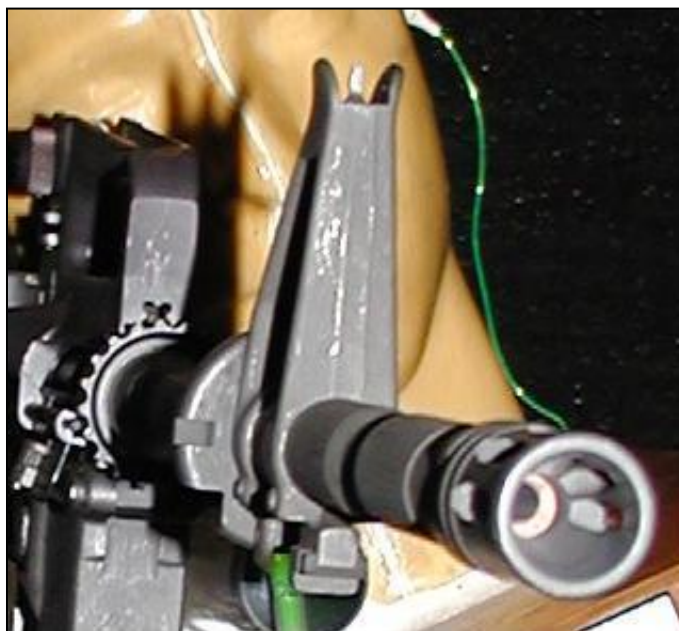
Figure 30. Muzzle compensator with asymmetric venting.
