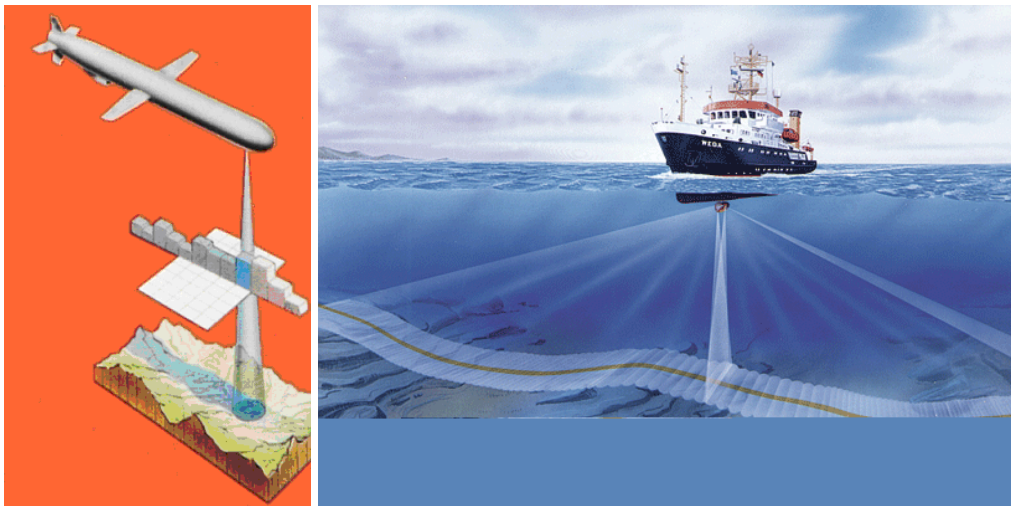
Figure 3-43: Terrain Referenced Navigation by Radar (left) and Sonar (right).
