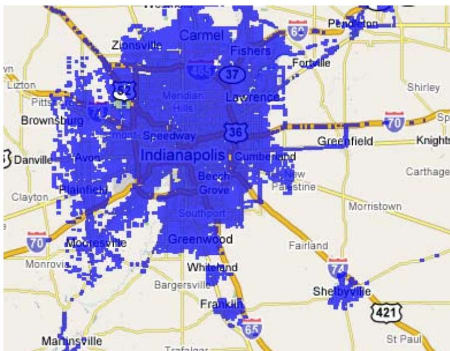
Figure 3-30: Known internet Wi-Fi hotspot locations near Indianapolis are exploited by the Wi-Fi positioning system being developed by Skyhook Wireless Inc.
