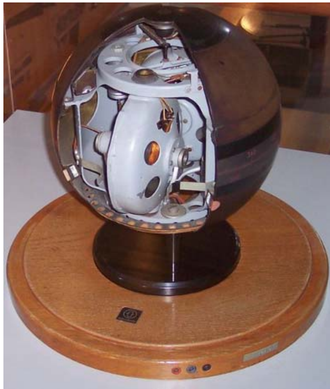
Figure 3-12: Cutaway of an Early Anschütz Gyrocompass (Wikipedia Commons Image).
