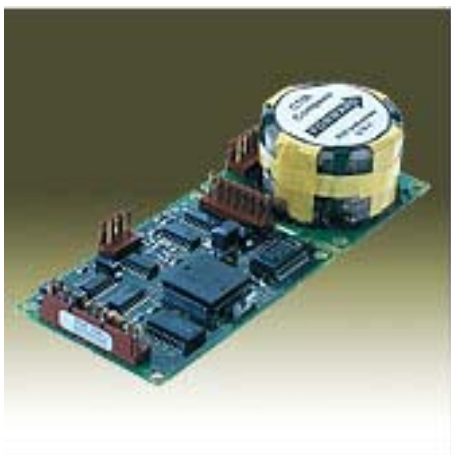
Figure 3-10: A Digital Magnetic Compass from KVH Industries.
