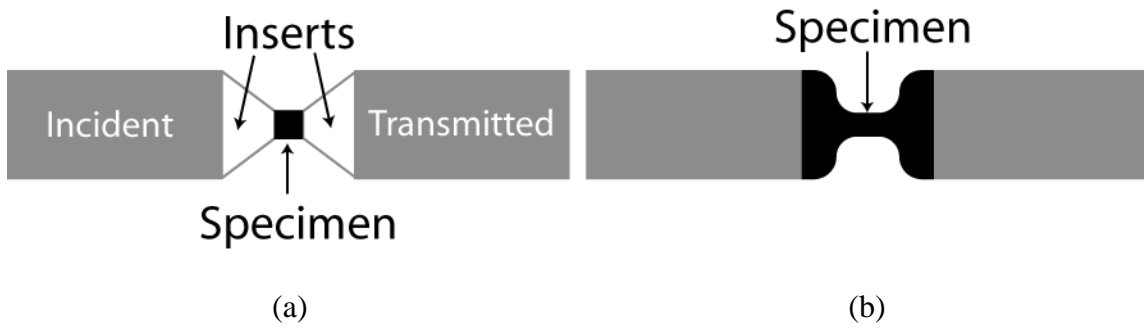
Figure 3.1 – Additional specimen geometries considered in testing low-ductility materials: (a) Conical inserts, (b) Dogbone compression specimen
