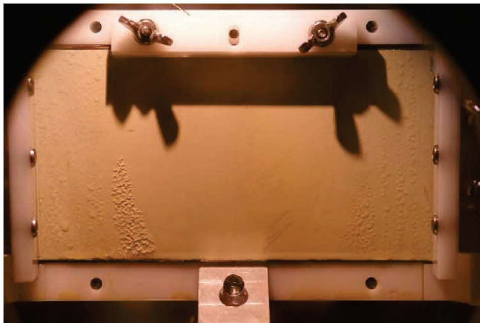
Figure 18. Old BMS 10-39 panel in the FTTP simulation box showing severe swelling after one day of exposure to vapors from 0.10 vol% DiEGME in the fuel.
