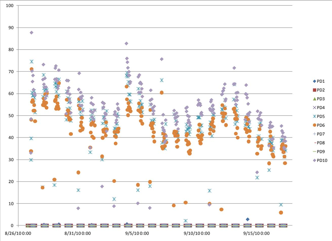
**Figure 5** Variations in bioluminescence intensity from a less photosensitive version of the bathyphotometer. Light levels were only recorded on those photodiodes that, by chance, had positive offsets – keeping the signal levels within the measurement range.
