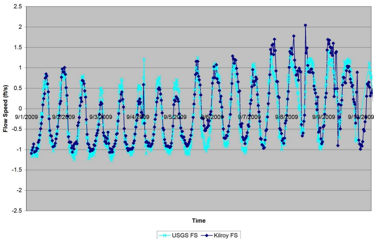
**Figure 4 Comparison between measurements from a USGS maintained flow meter in Jewfish creek, north of Key Largo, Florida and collocated Kilroy acoustic travel time flow meter from Sept. 1-10, 2009. Light blue data points in background are from the USGS sensor, while darker blue points in the foreground are from the Kilroy acoustic flow meter.**
