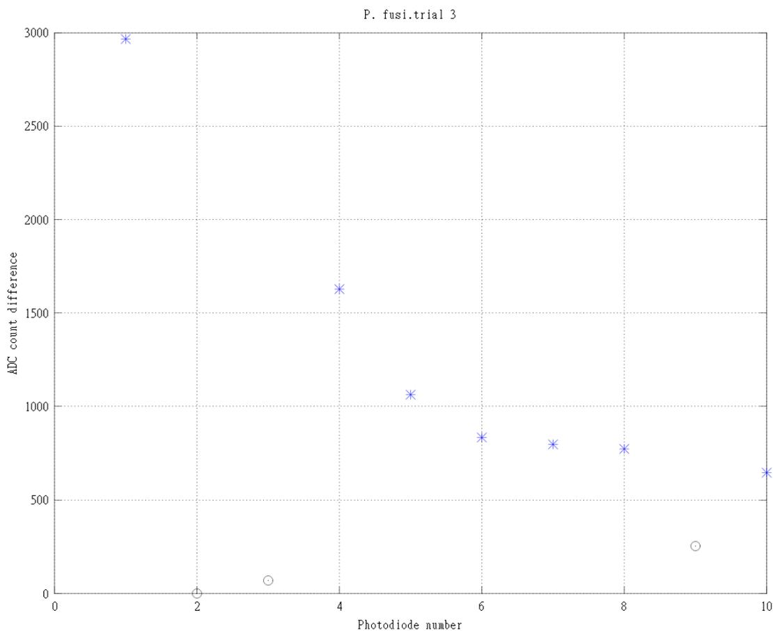
**Figure 5** *Bioluminescence intensities from Pyrocystis fusiformis in laboratory tests of bathyphotometer. Photodiode number 1 is closest to the point of excitation. Circles indicate dysfunctional photodiodes.*
