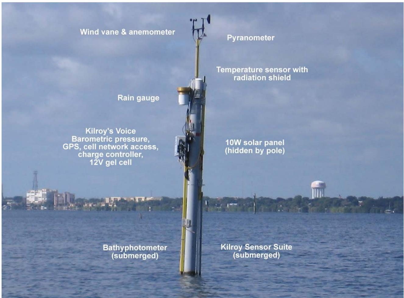
***Figure 3 Kilroy Network station deployed west of Cocoa, Florida. Station consists of a complete meteorological station, Kilroy sensor suite, bathypotometer, Kilroy's Voice cellular Internet gateway, a 12 Ah, 12V gel cell battery, charge controller, and 10W solar panel.***
