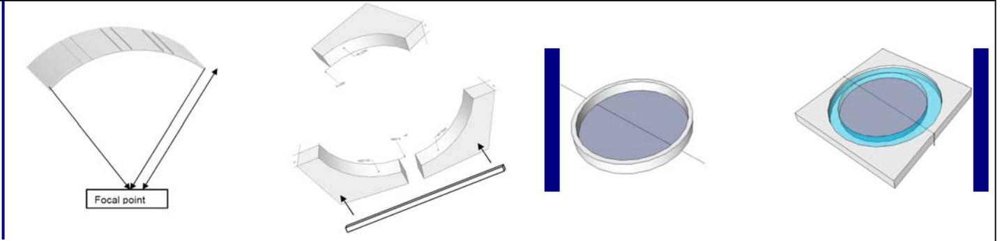
Fig 5: A **preliminary array design study** has centered on 2-4 interlocking modular sections of a backed PZT 1-3 composite for straightforward positioning around the head. Insertable gel-based and water-filled membranes will be considered for optimal coupling. Our ongoing human subject study during brain surgery has confirmed the ability to transmit via shear mode windowing, and to couple US through hair using US gel.
