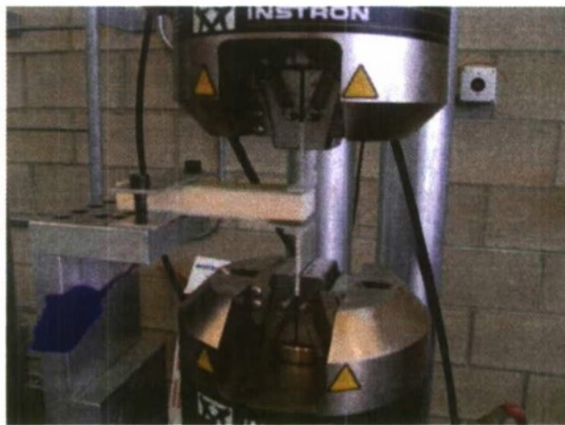
Figure 45 - 100 kN load cell Instron grip configuration
