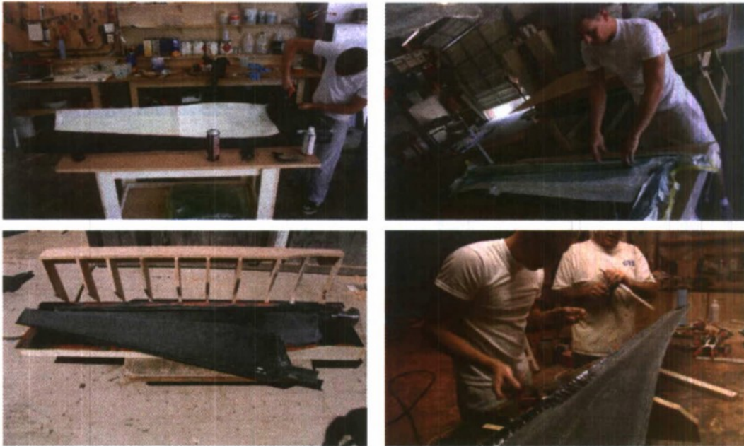
FIGURE 3: FOUR OF THE STEPS DEVELOPED IN THE BLADE MANUFACTURING PROCESS. CLOCKWISE, FROM TOP LEFT: MOLD LAY-UP OF FIBERGLASS CLOTH; VACUUM BAG SETUP FOR ONE HALF OF THE BLADE; GLUE PREPARATION OF THE CURED HALF; ASSEMBLY OF TWO CURED HALF BLADES IN A CUSTOM CLAMPING JIG. THE LAY-UP SCHEDULE ITSELF IS A CRITICAL STEP THAT REQUIRED EXTENSIVE ANALYSIS AND TEST. NOTE THAT CLIPPER WINDPOWER PARTICIPATED IN THE CRITICAL DESIGN REVIEW OF THIS PROCESS; THE FINAL METHOD DEVELOPED IS SIMILAR TO THAT USED IN THE UTILITY-SCALE BLADE MANUFACTURING INDUSTRY.
