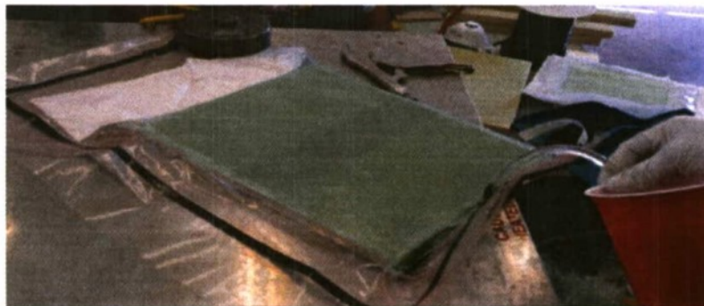
Figure 36 - VaRTM composite lay-ups resin flow
