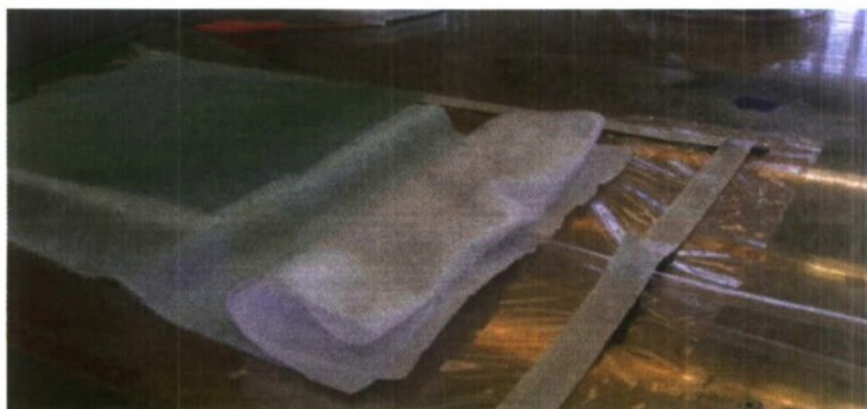
Figure 33 - Stacked VaRTM lay-up before vacuum bagging
