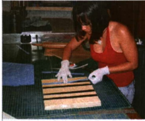
Figure 43 - DADs being inserted into foam slots
