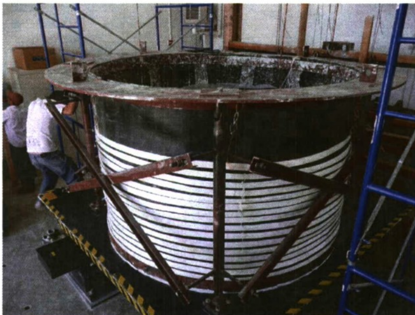
Figure 5. Full barrel being prepared for initial calibration tests. Notice cross braces are still in place and will be removed prior to testing to allow the flexible barrel free movement in response the imposed seismic shaking.
