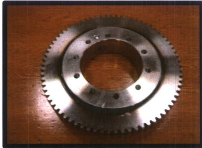
Figure 6.2.1.2: Image of the Gear Tek swing bearing used in the WTN
