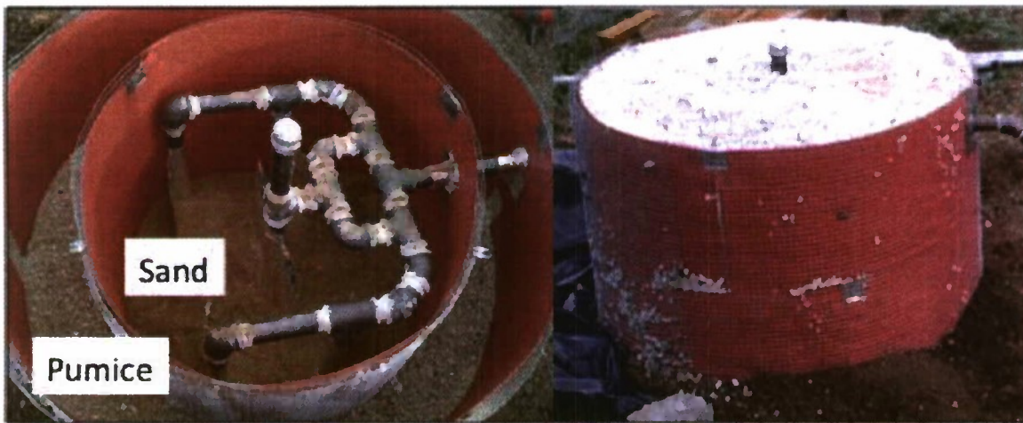
Fig. 2a) The solar thermal storage facility from above ( left ) before being filled with sand and pumice. The outer cylinder is full of pumice as an insulator. The center cylinder is filled with sand, which stores the heat. The heat is distributed throughout the center by means of pipes containing motor oil. Right , After being filled with sand, the top surface of the storage unit was covered with more pumice for insulation.
