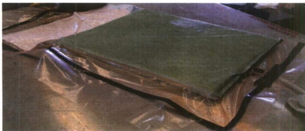
Figure 34 - Vacuum bagged composite sandwich structure after lay-up
