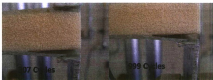
Figure 68 - 1.0 inch delamination fatigue crack propagation through foam
