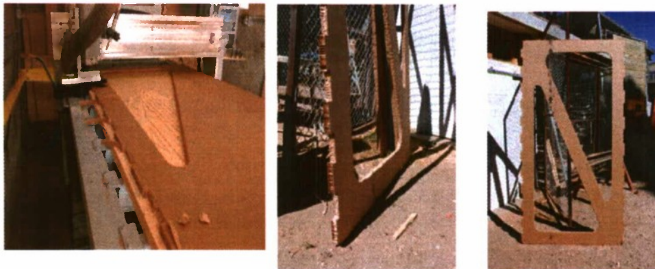
Figures 14a-c. Using a CNC router to cut all corrugated paperboard components of prototype 5
