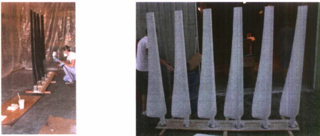
FIGURE 4: THE BLADES ARE PROTECTED WITH A POLYURETHANE-BASED PAINT.
