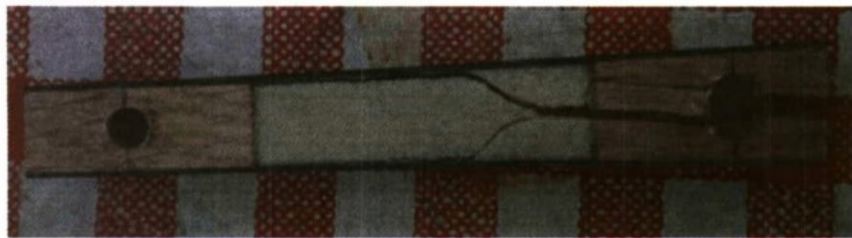
Figure 101 - Failure of overall material property specimens
