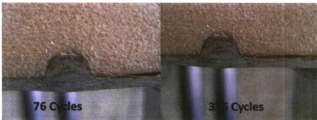
Figure 71 - Shear key fatigue failure analysis
