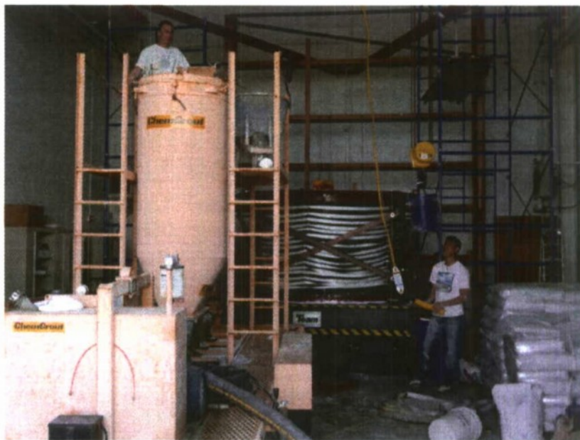
Figure 3. Testing platform showing the shake table with the flexible wall barrel installed. The flexible wall barrel is composed of the four corner posts with universal joints at the top and bottom, top and bottom rings, and the barrel wall. The wall is composed of a 6.4 mm thick rubber membrane which is confined by 45 mm wide Kevlar straps spaced on center every 60 mm. The (yellow) mixer on the left is used to mix large volumes of model soil (composed of kaolinite, bentonite, fly ash, and water) for filling the barrel.
