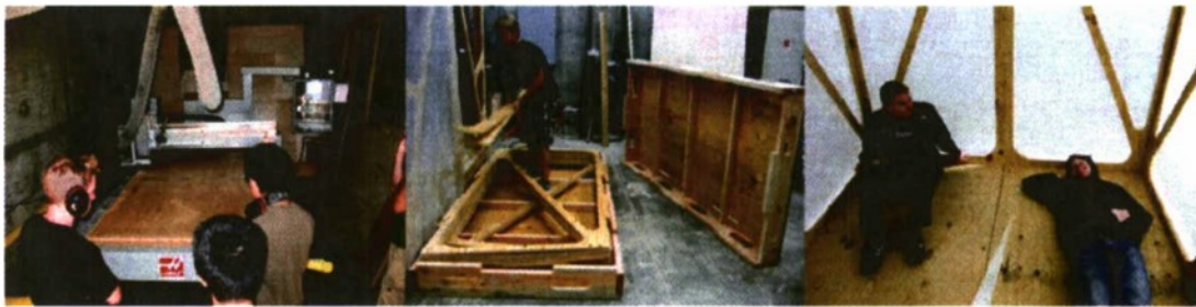
Figures 13a-c. Using a CNC router to cut all components of prototype 4 (a, left), the floor is used as a packing crate for wall and roof components (b, center), and the interior of prototype 4 (c, right).
