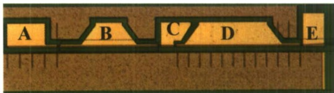
Figure 1. This is a top view of a single-chip Sampled Grating Distributed Bragg Reflector Laser (SGDBR) used for OCT measurements. Currents in Back Mirror (A), Front Mirror (D), and Phase Section (C), control the laser frequency. Currents in the gain section (B) and the semiconductor optical amplifier (E) control the laser power. The chip dimensions are 0.5 mm by 3 mm.
