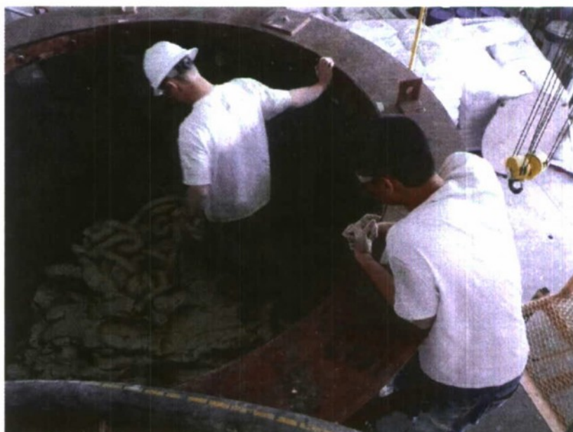
Figure 4. Process of filling the barrel with scale model soil is shown. Ten accelerometers were placed within the soil in both vertical and horizontal arrays to measure the dynamic response of the soil during seismic shaking.
