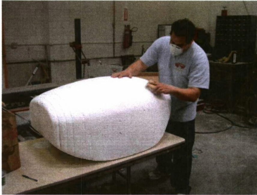
Figure 6.3.2: Alvaro Martinez shaping the foam plug of the fairing to be used for the WTN.
