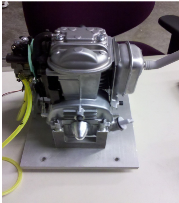
Figure 38: Honda GX-35 engine with prop nut on shaft for starting
