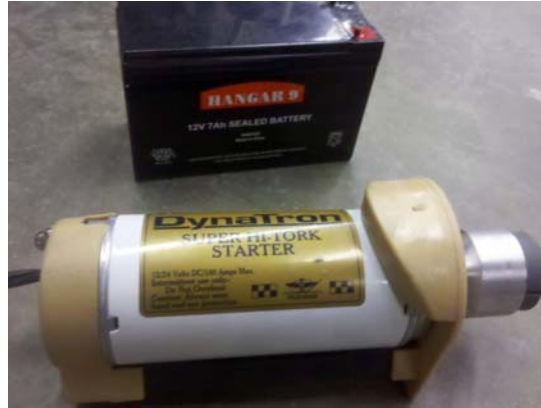
Figure 37: Sullivan DynaTron Hi-Torque starter [52] with 12V power battery
