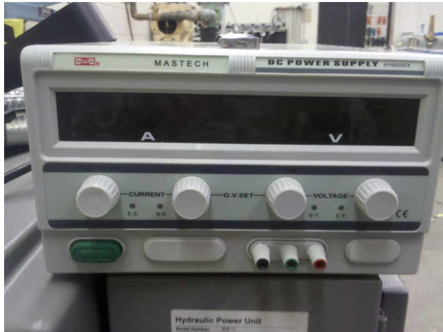
Figure 35: Mastech DC power supply
