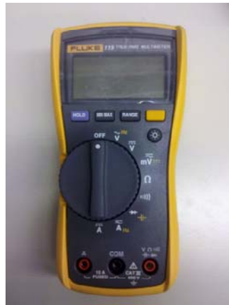
Figure 52: Fluke Model 115 True-RMS Multimeter used for current and voltage measurements
