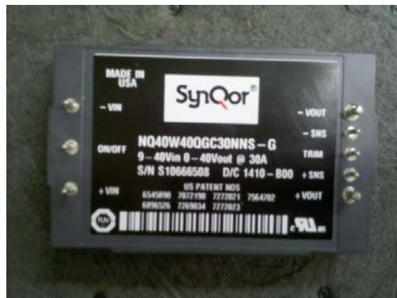
Figure 34: DC/DC Converter being used for both propulsion and generation
