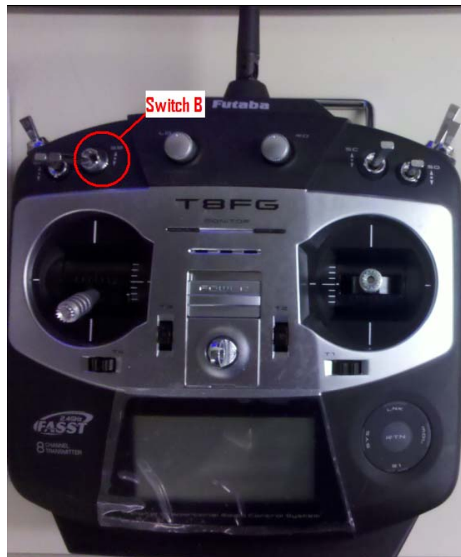
Figure 21: Transmitter depicting switch B.
