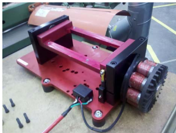
Figure 32: Dynamometer without any mounted equipment; note mounted strain gauge for torque measurement
