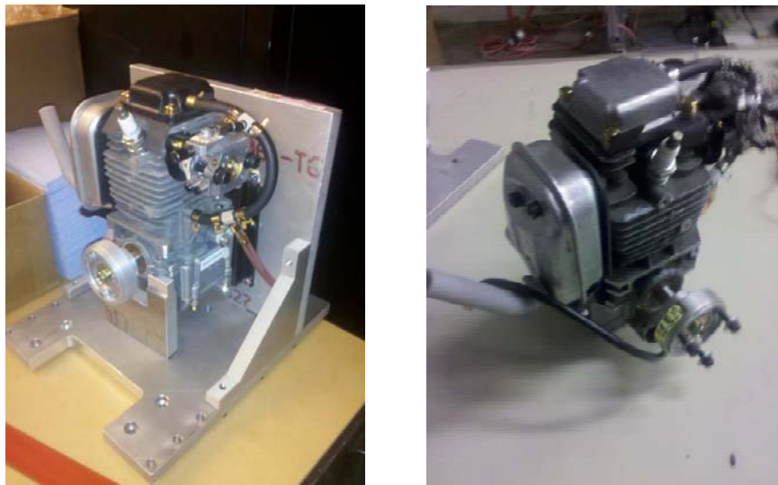
Figure 36: Fuji BF25-EI with mounting brackets (left) and BF34-EI (right) from the bottom due to negative experiences with mounting engines from the backplate. The Honda is rated for a maximum of 1.3 HP and also runs on 87 grade automotive gasoline.
