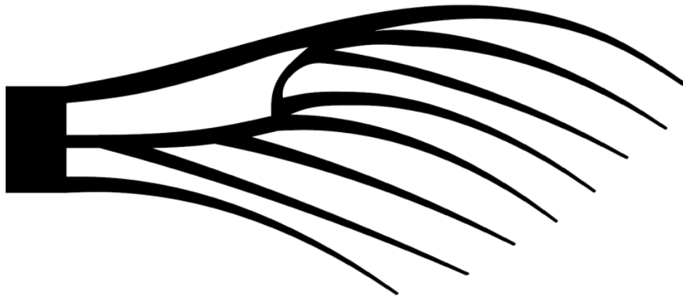
Figure 19: CAD program is used to make a representation of the wing that can be used to make the fabrication mask
