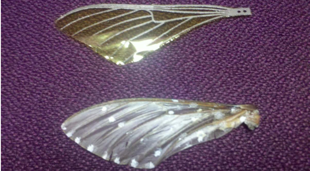
Figure 53: Manufactured wing side by side with a hawkmoth wing shows they are indeed similar in size and structure
