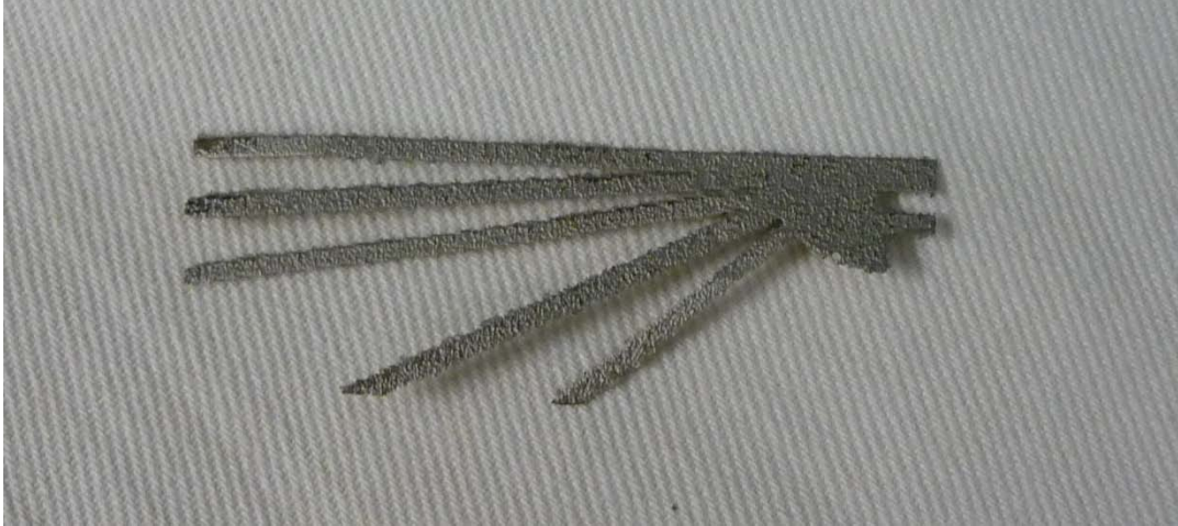
Figure 36: Surface of initial stylized wing was rough due to partially exposed positive photoresist
