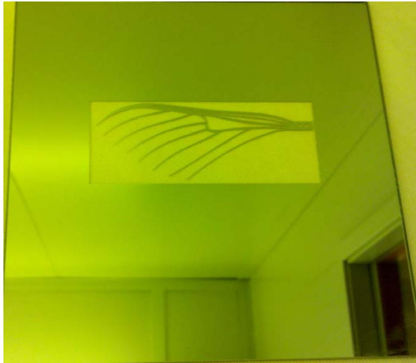
Figure 23: Finished mask of final wing design, chrome on soda lime, taken in cleanroom (hence the yellow light) to avoid dust contamination
