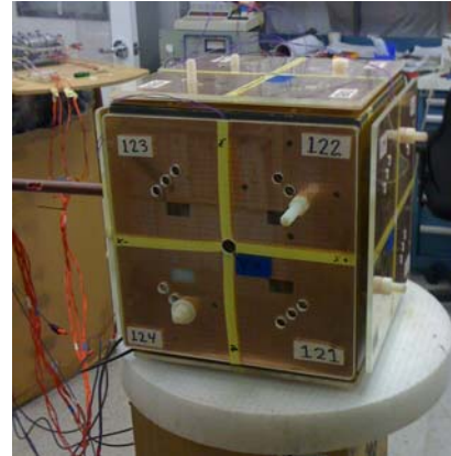
Figure 1. LBNL Hand-held UXO Discriminator - (a) transmitter-receiver array configuration, (b) assembled prototype.
