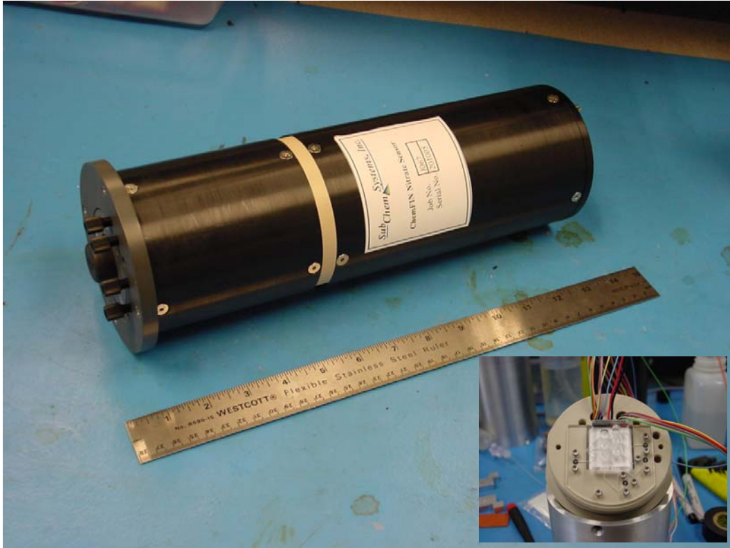
Figure 1. SubChem Systems's compact design for ChemFIN™ the next generation chemical sensing payload for AUVs, Gliders and Profilers. The ChemFIN compact microfluidics module is also shown (inset).
