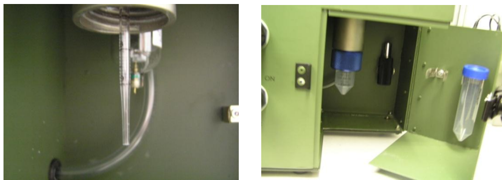
Figure 8: XMX impinger module with (right) and without (left) collection tube (Cooper, 2010)
