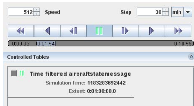
Figure 89: Time Control with buttons to disable or pause each controlled table
