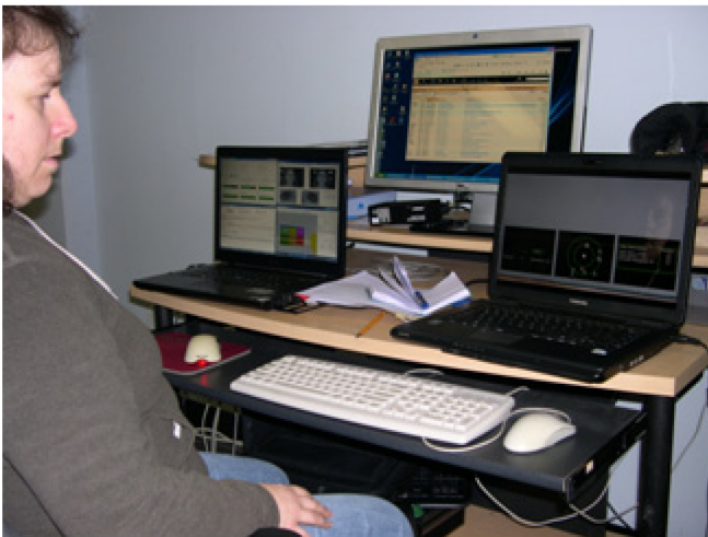
Figure A-11: The two laptops used. L1 on left (controlled faceLAB). L2 on right controlled presentation software (Python). Computer in back (LCD) was used for data analysis (but not used during the experiment).
