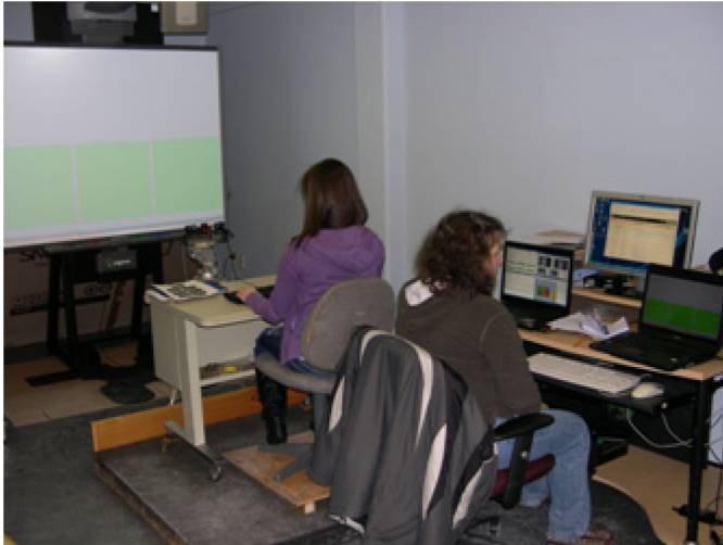
Figure A-10: Entire set-up from a distance (calibration step). Participants were in a raised chair in front of faceLAB cameras. Experimenter at desk in front of laptops (the ‘experimenter’ in this photo was not the actual experimenter but an RA posing as the experimenter).
