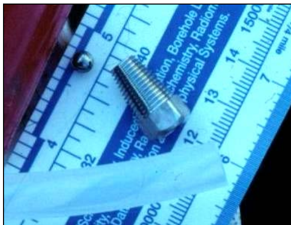
Figure 8. Equipment used to redevelop wells, including small check valve, check ball, and poly-tubing used to redevelop smaller DP wells.
