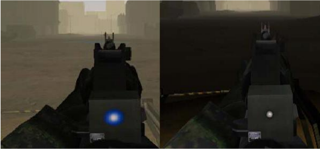
Figure 3. Rifle-mounted IFF device used in Experiment 1, which blue light on to indicate friend and unlit to indicate not-a-friend.
