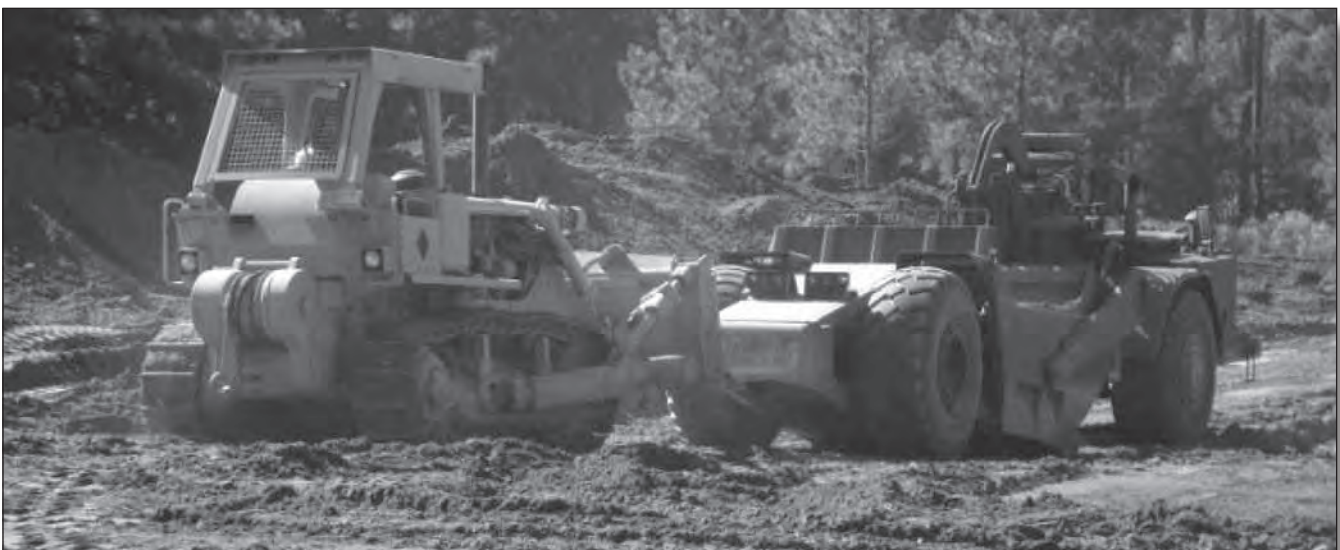
A Soldier uses a D7 bulldozer to push-load a scraper.
