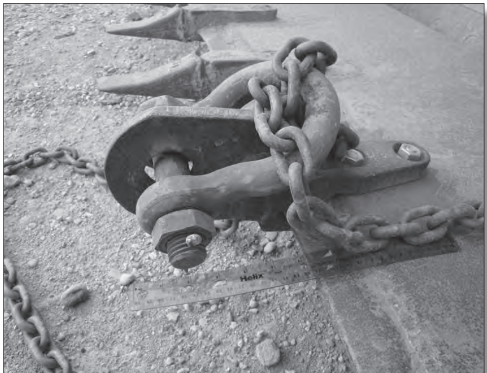
A clevis and chain turn a bucket loader into a device to maneuver Jersey barriers.
