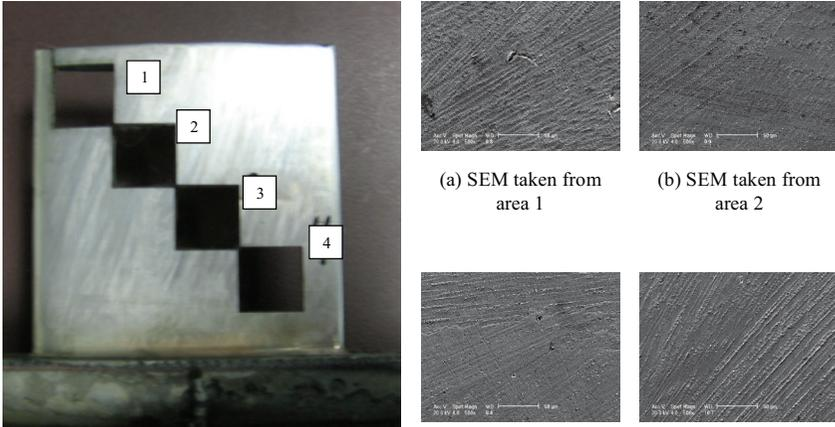
Figure 8. Surface texture of generic airfoil (material: IN625, ~2" wide, ~2" high)
