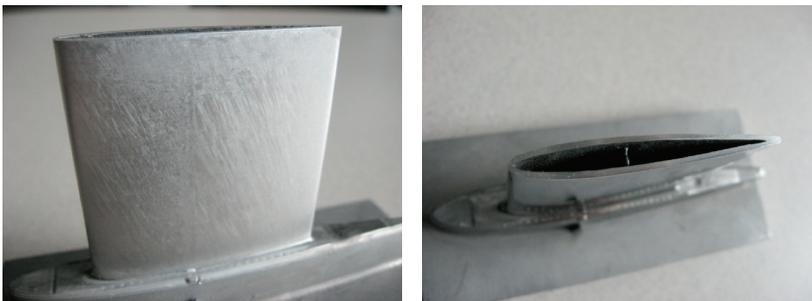
Figure 7. (a) Front view of generic airfoil (IN625) showing interrupted DS texture due to grinding of the layered surface, (b) Top view of the airfoil
