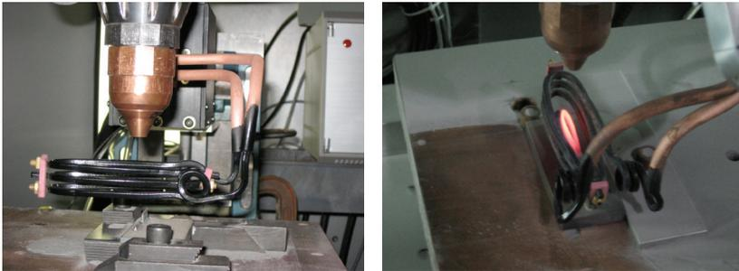
Figure 9. Induction system assembled with DMD process
