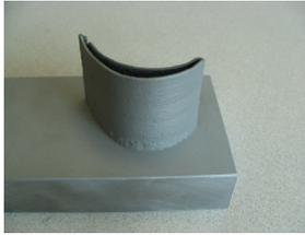
Figure 4. Partially finished turbine blade (Material: IN625)
