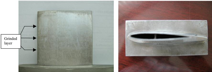
Figure 6. (a) Front view of generic airfoil (IN718) showing interrupted DS texture due to grinding of the layered surface, (b) Top view of the airfoil
