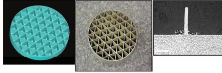
Figure 1. Serpentine cooling channel of blade      Figure 2. Sample with fine resolution (Wall thickness = 0.26 mm, Material: IN625)
