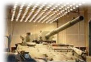
Environmental Test Cell
