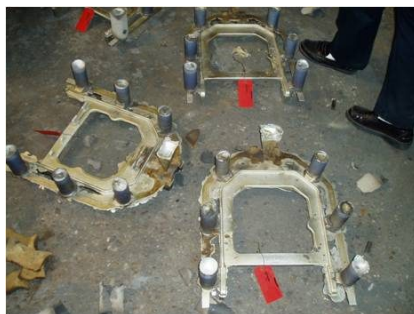
(b) seat frame castings after shake-out
