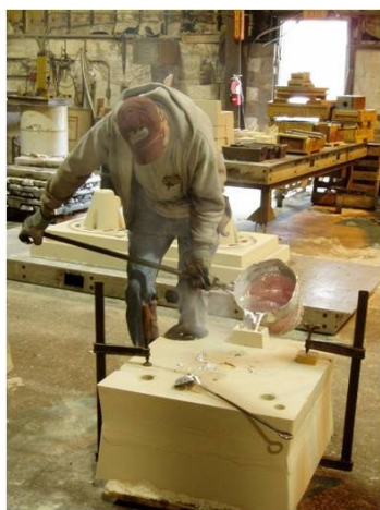
(a) seat frame casting being poured
