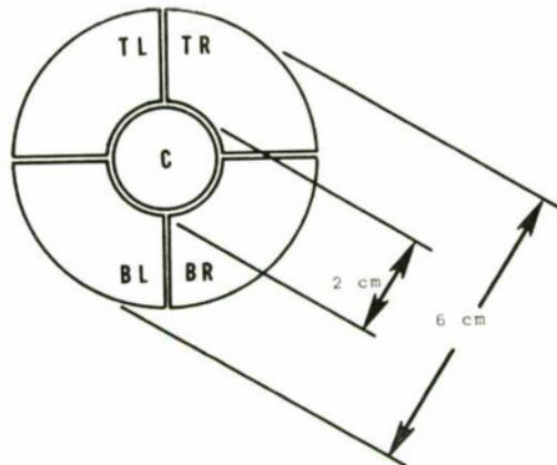
Figure 4. Experimental target, divided into a centre segment and a four-part outer ring.
