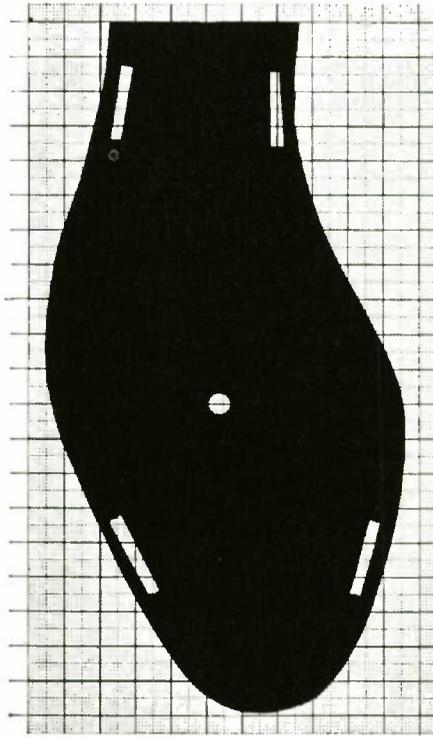
Figure 3. Experimental sandal: Partial sole made of 0.4 cm fibreboard. The sketch (on a 1 cm  $\times$  1 cm grid) shows the location of the brass spike (protruding 2 cm downward, diameter at the end 0.5 cm) and of slots for straps to attach the sandal to the subject's foot.
