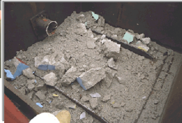
Figure 3. In-Water Test of 4' Cube (top exposed to air) with 203 mm Cu SR
