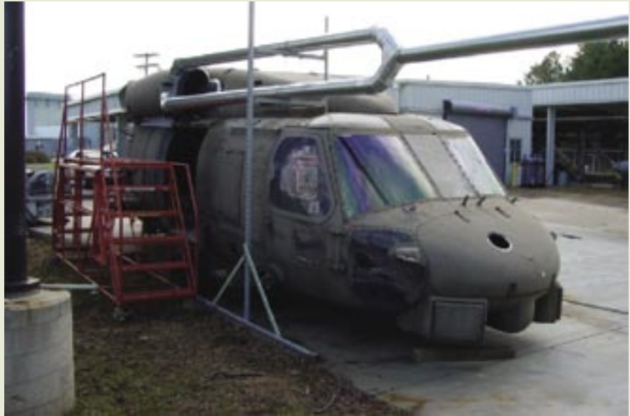
Figure 3. H-60 Engine Nacelle Test Setup
