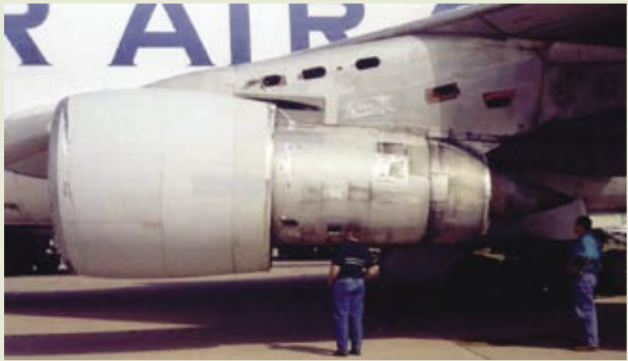
Figure 3. JT9D Engine for MANPADS Test
