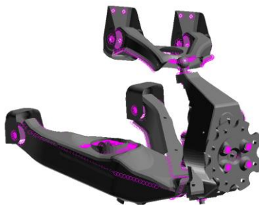
Fig. 1. Schematic of the double A-Arm suspension of HMMWV
