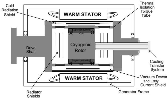
Fig. 2. Basics of a classic superconducting generator.
