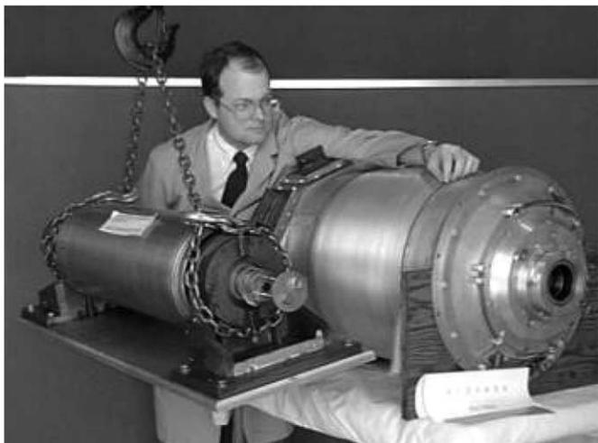
Fig. 3. Superconducting NbTi-based 5 MW generator, circa 1974, resulting from an Air Force contract with Westinghouse.
