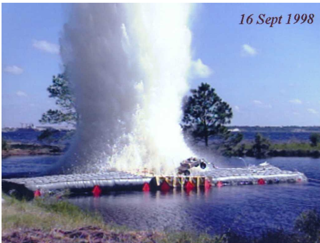
Figure 2. Assembled Foam Bridge Subjected to Nearby Explosion
