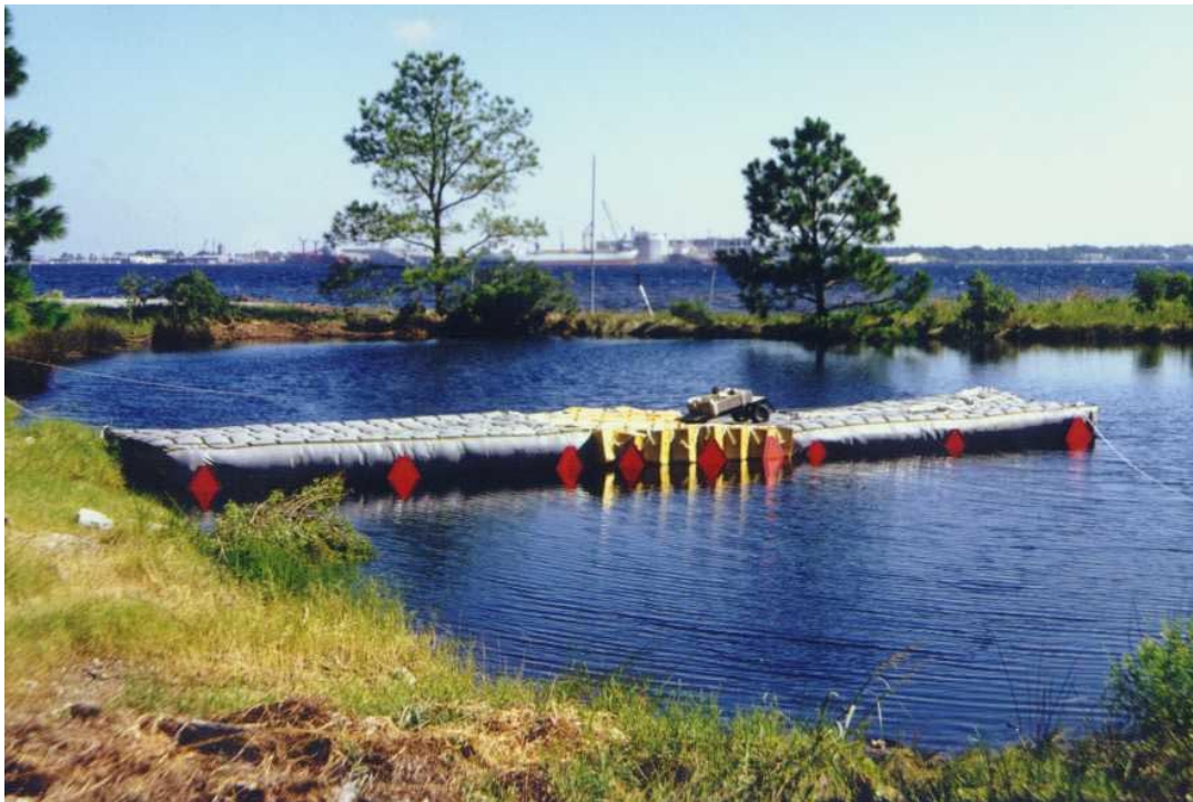
Figure 1. Assembled Foam Bridge at CSS Test Pond
