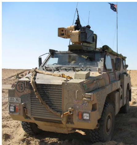
Figure 2. A modified Bushmaster PMV with CROWS Remote Weapon Station in Iraq during 2008
