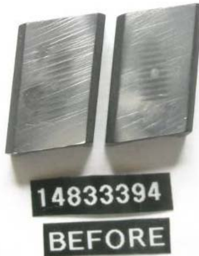
Figure 29 - Pump SN: 14833394 Roller Shoe Condition before Testing with R8 + 22.5-ppm DCI-4A Fuel
