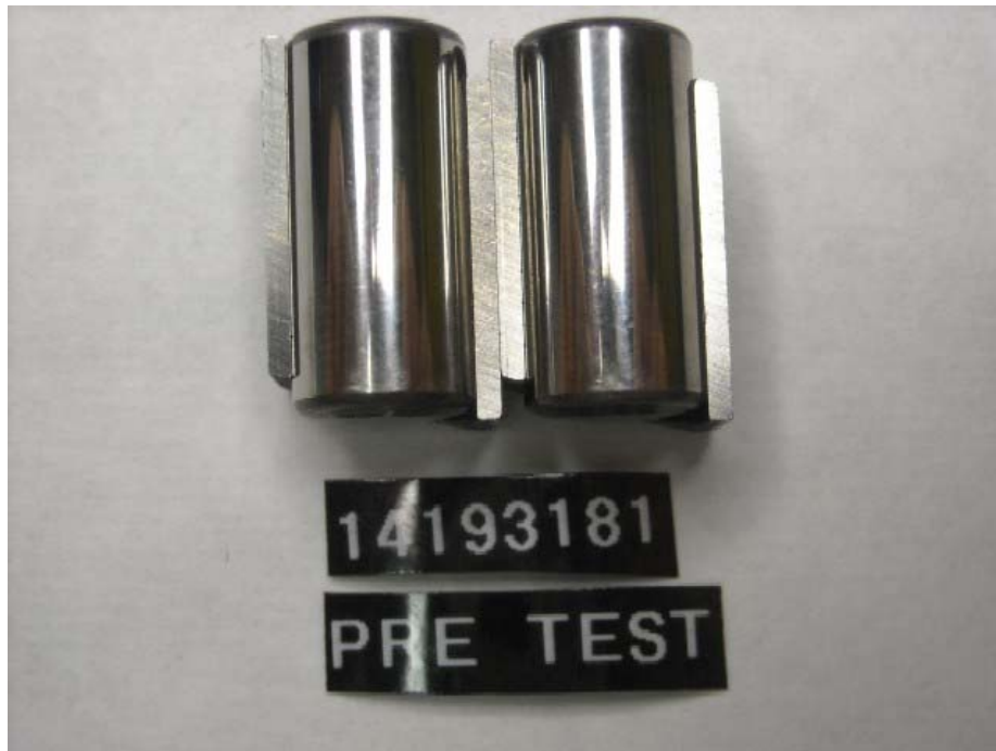
Figure I-1-37. Injection Pump SN:14193181 Pre-Test Roller Shoes and Rollers
