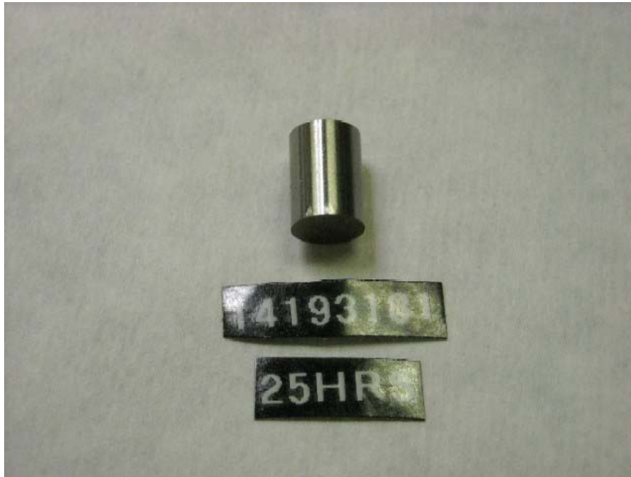
Figure I-1-53. Injection Pump SN:14193181 Transfer Pump Regulator Piston Wear
