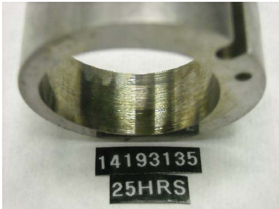
Figure I-1-27. Injection Pump SN:14193135 Transfer Pump Liner Wear
