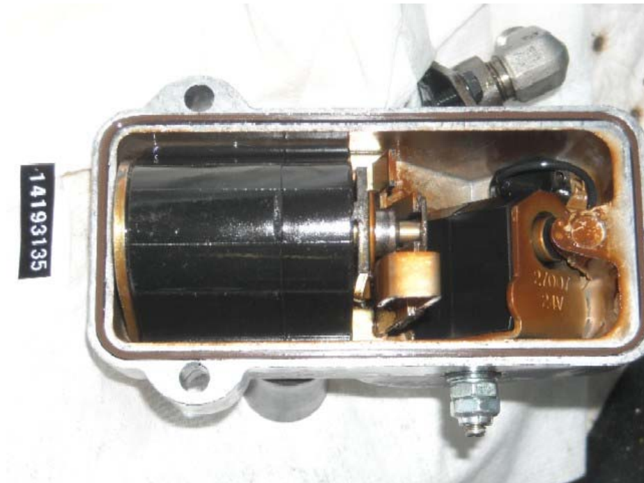
Figure I-1-8. Injection Pump SN:14193135 Top Cover with Disposition and Wear Debris
