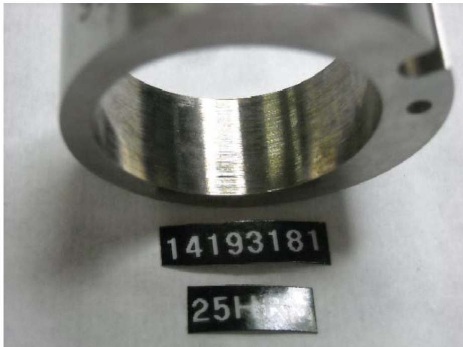
Figure I-1-48. Injection Pump SN:14193181 Transfer Pump Liner Wear
