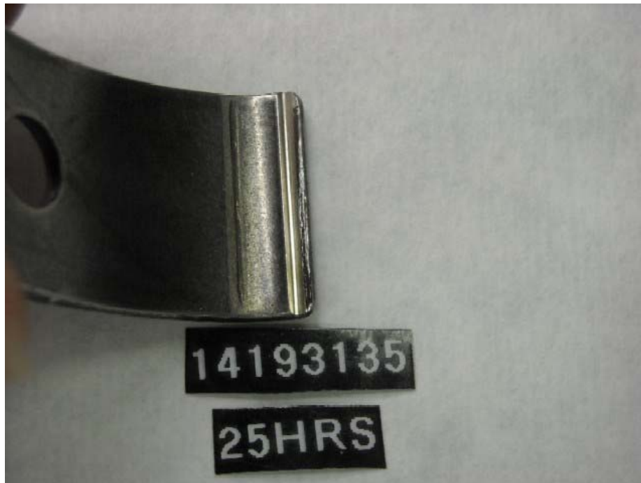
Figure I-1-18. Injection Pump SN:14193135 Leaf Spring/Roller Shoe Wear Contact
