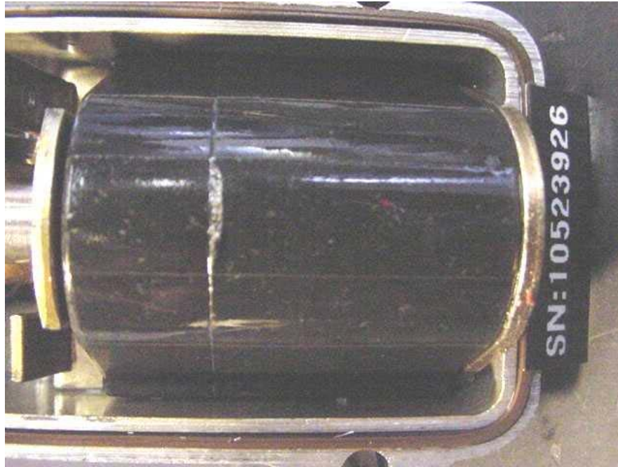
Figure I-1A-4. Test 1 Pump 2: Debris Free Solenoid
