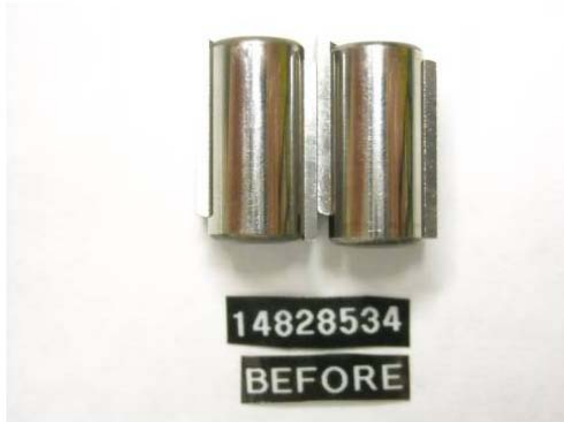
Figure 43 - Pump SN: 14828534 Rollers and Shoe before Testing with R8/JET-A + 22.5-ppm DCI-4A Fuel
