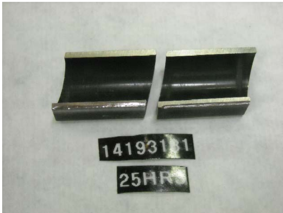
Figure I-1-40. Injection Pump SN:14193181 25-Hour R-8 Fuel Roller Shoes
