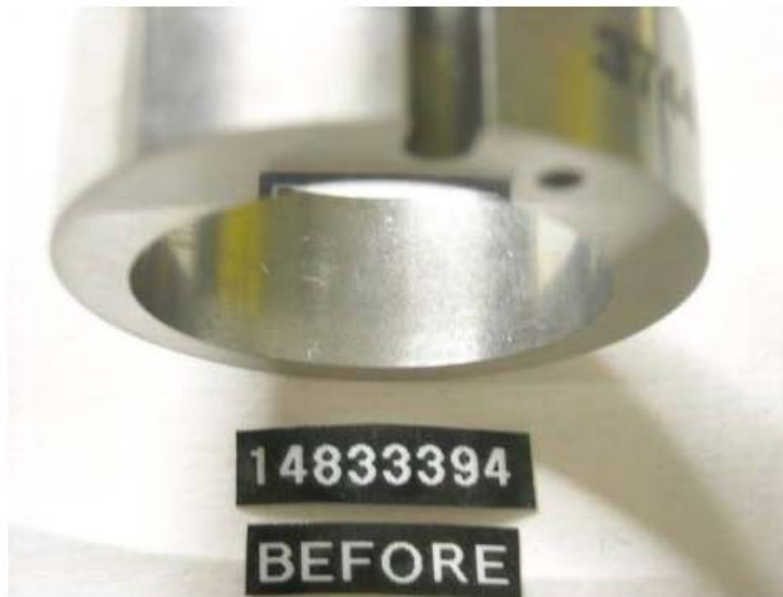
Figure 35 - Pump SN: 14833394 Transfer Pump Liner before Testing with R8 + 22.5-ppm DCI-4A Fuel
