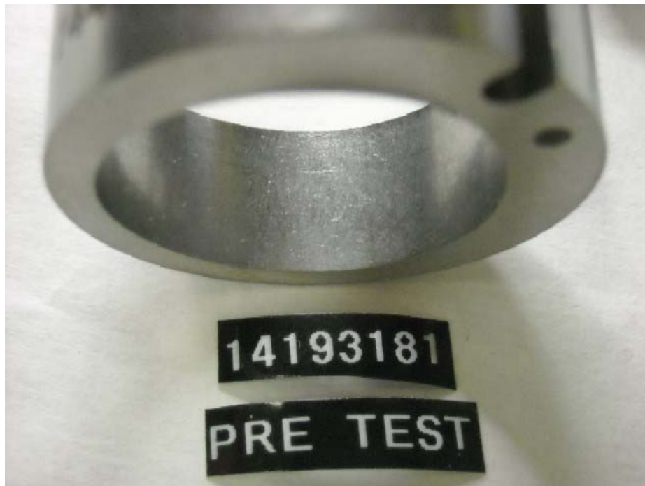
Figure I-1-47. Injection Pump SN:14193181 Transfer Pump Liner Pre-Test Condition
