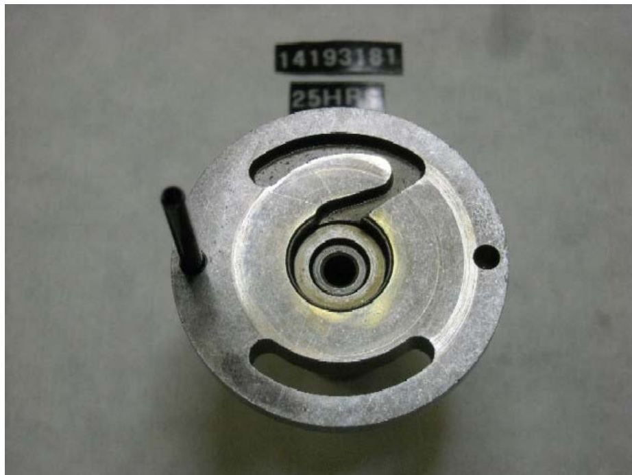
Figure I-1-52. Injection Pump SN:14193181 Transfer Pump Regulator Wear
