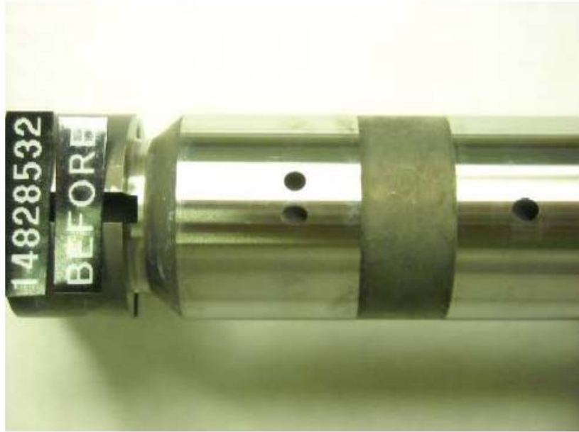
Figure 9 - Pump SN: 14828532 Distributor Rotor before Testing with R8 + 22.5-ppm DCI-4A Fuel
