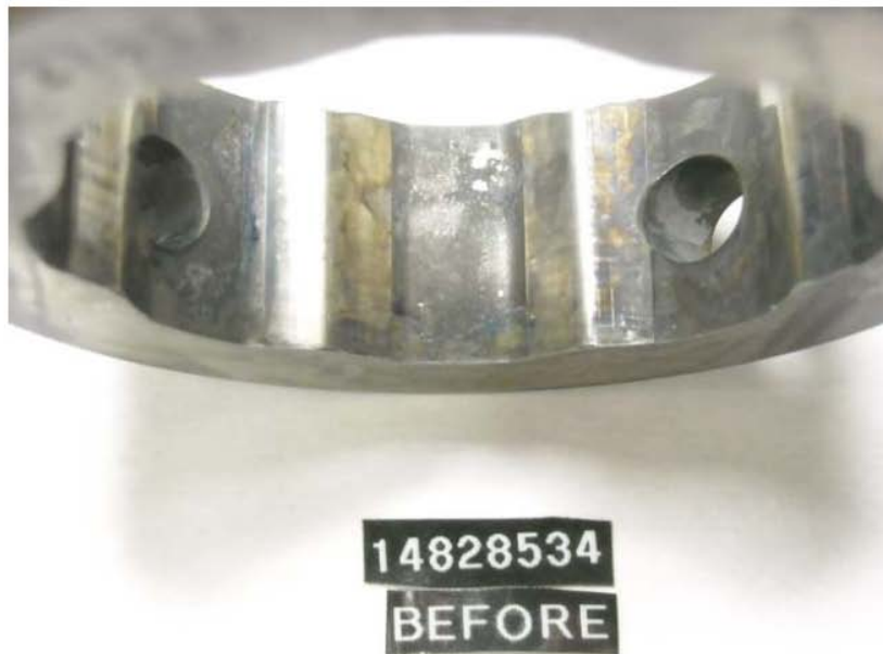
Figure 47 - Pump SN: 14828534 Cam Ring before Testing with R8/JET-A + 22.5-ppm DCI-4A Fuel
