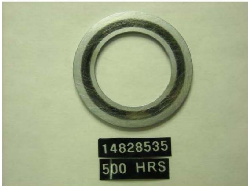
Figure 66 - Pump SN: 14828535 Thrust Washer with 500-Hours Testing with R8/JET-A + 22.5-ppm DCI-4A Fuel
