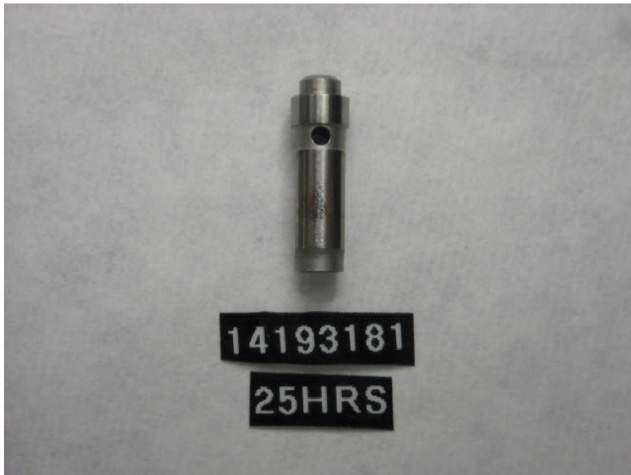
Figure I-1-36. Injection Pump SN:14193181 Delivery Valve Wear Scar
