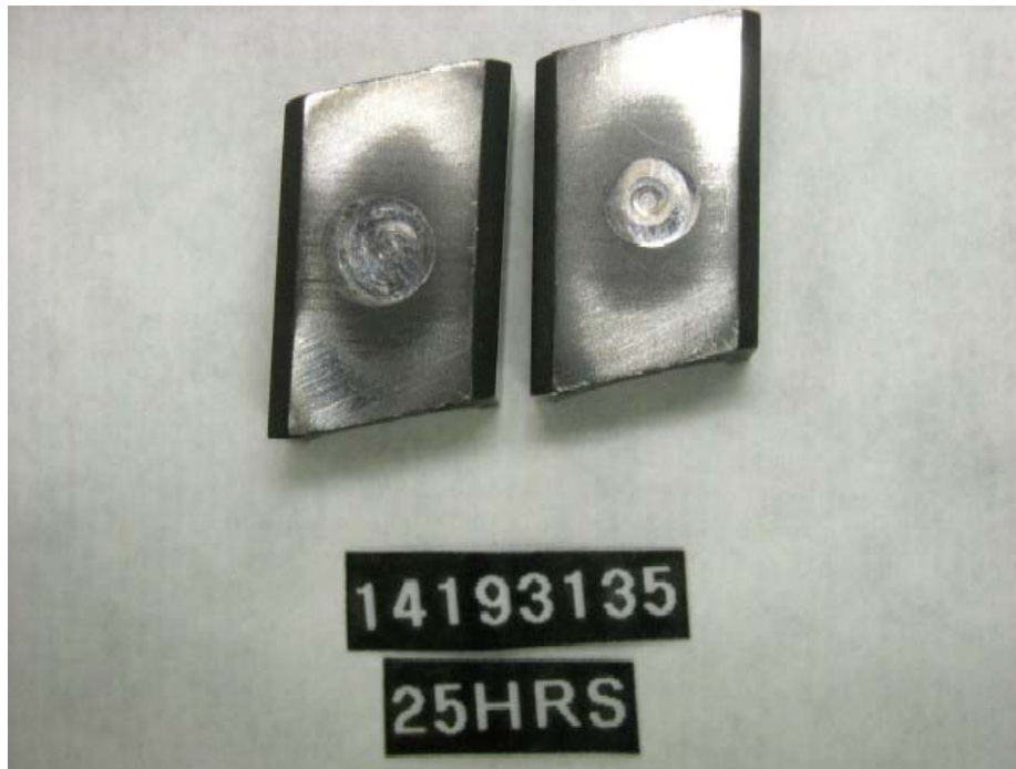
Figure I-1-20. Injection Pump SN:14193135 Roller Shoe Plunger Contacts
