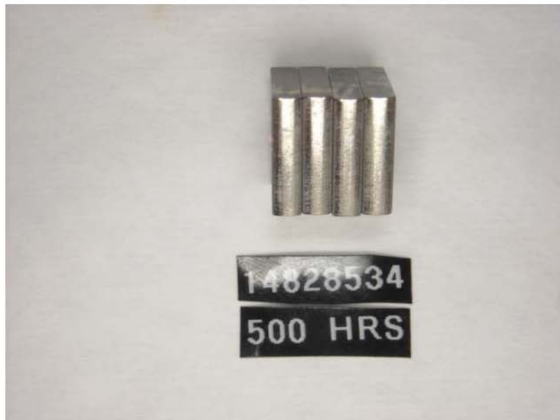
Figure 54 - Pump SN: 14828534 Transfer Pump Blade Edges with 500-Hours Testing with R8/JET-A + 22.5-ppm DCI-4A Fuel
