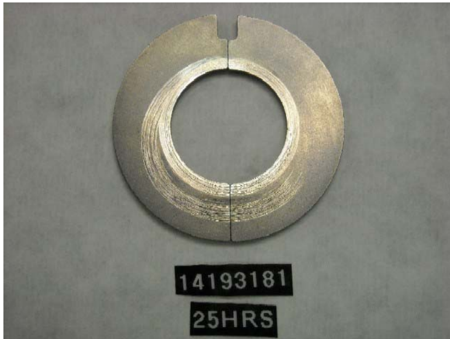
Figure I-1-51. Injection Pump SN:14193181 Rotor Retainer Wear
