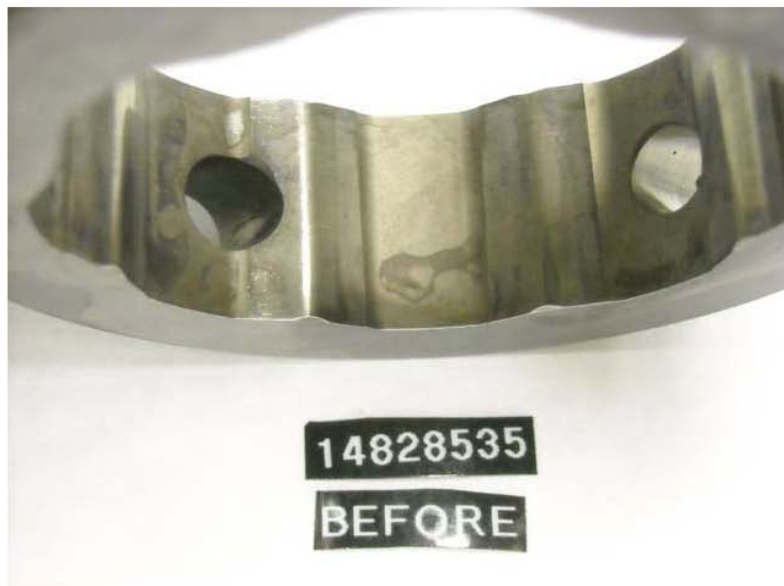
Figure 63 - Pump SN: 14828535 Cam Ring before Testing with R8/JET-A + 22.5-ppm DCI-4A Fuel
