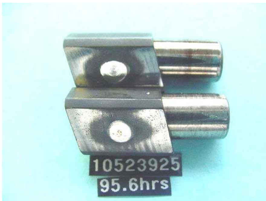
Figure I-1A-7. Test 1 Pump 1: Shoe Back and Roller Wear
