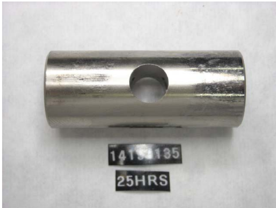
Figure I-1-24. Injection Pump SN:14193135 Advance Piston Wear
