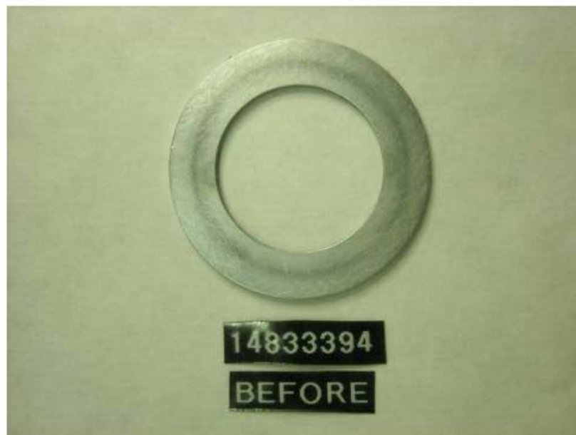
Figure 33 - Pump SN: 14833394 Thrust Washer before Testing with R8 + 22.5-ppm DCI-4A Fuel
