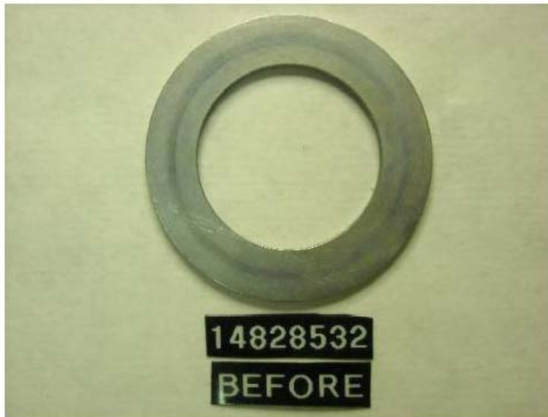
Figure 17 - Pump SN: 14828532 Thrust Washer before Testing with R8 + 22.5-ppm DCI-4A Fuel
