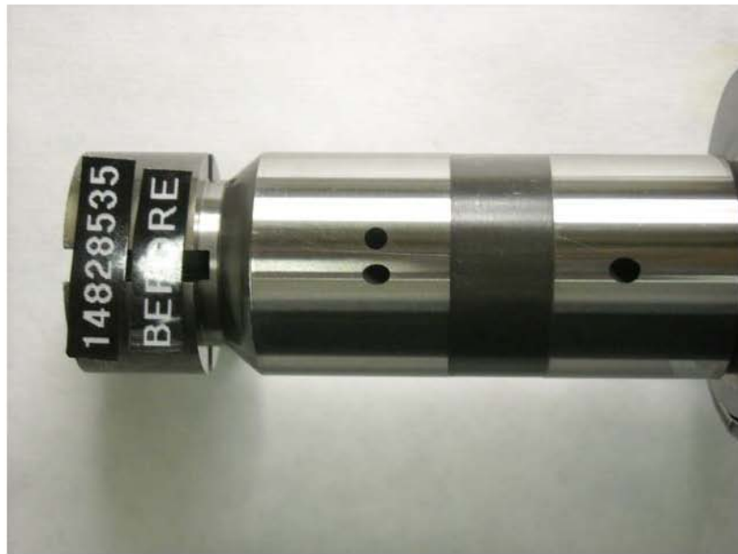
Figure 57 - Pump SN: 14828535 Distributor Rotor before Testing with R8/JET-A + 22.5-ppm DCI-4A Fuel
