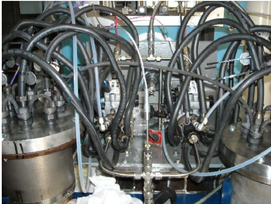
Figure I-1-3. Both R-8 Stanadyne Rotary Fuel Injection Pumps Mounted on Stand with Fuel Injectors
