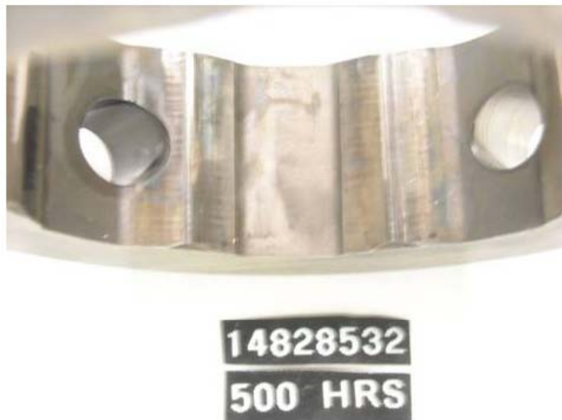
Figure 16 - Pump SN: 14828532 Cam Ring with 500-Hours Testing with R8 + 22.5-ppm DCI-4A Fuel
