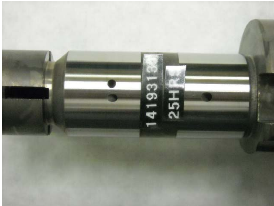
Figure I-1-13. Injection Pump SN:14193135 Rotor Discharge Ports with Minimal Wear
