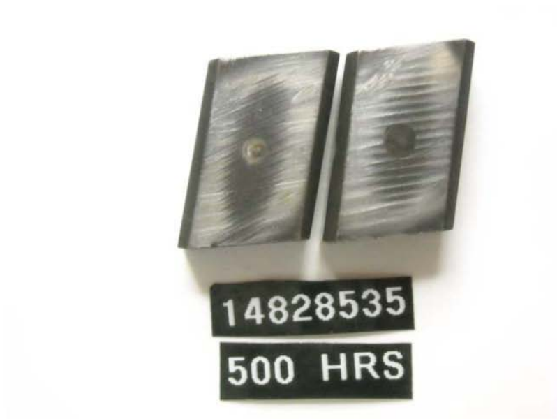
Figure 62 - Pump SN: 14828535 Roller Shoe with 500-Hours Testing with R8/JET-A + 22.5-ppm DCI-4A Fuel
