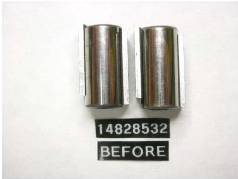
Figure 11 - Pump SN: 14828532 Rollers and Shoe before Testing with R8 + 22.5-ppm DCI-4A Fuel
