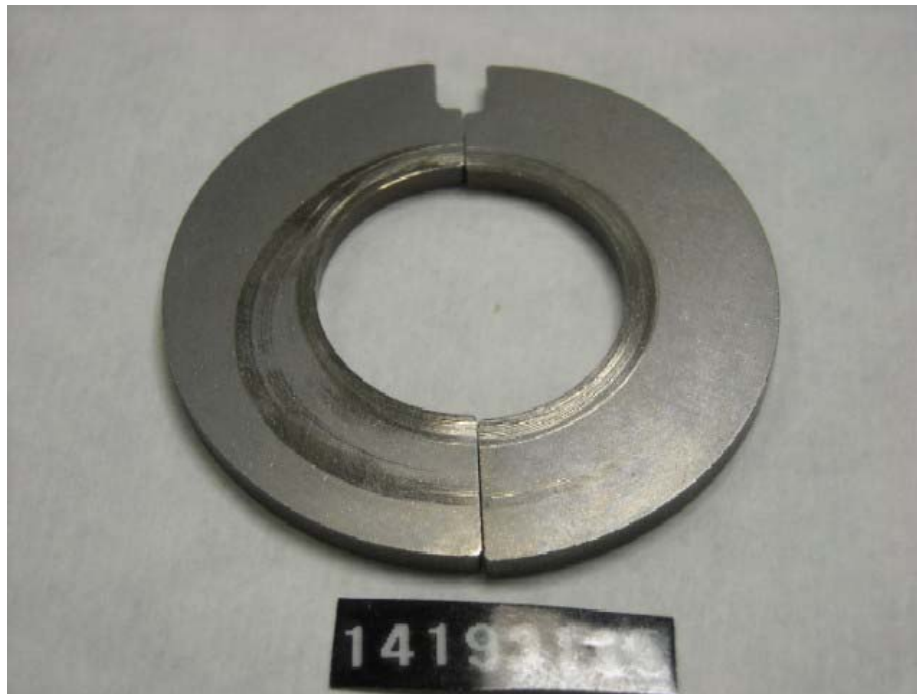
Figure I-1-30. Injection Pump SN:14193135 Rotor Retainer Wear
