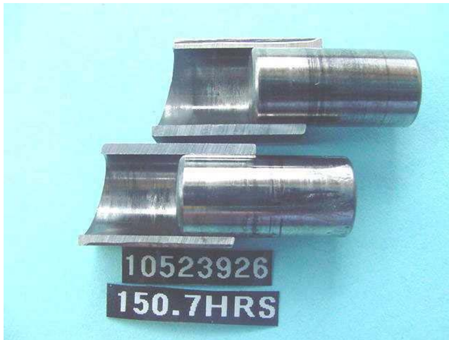
Figure I-1A-6. Test 1 Pump 2: Shoe and Roller Wear
