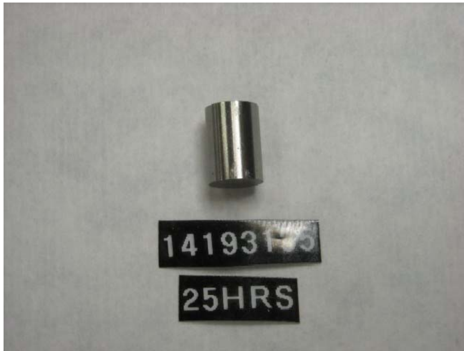
Figure I-1-32. Injection Pump SN:14193135 Transfer Pump Pressure Regulator Piston Wear
