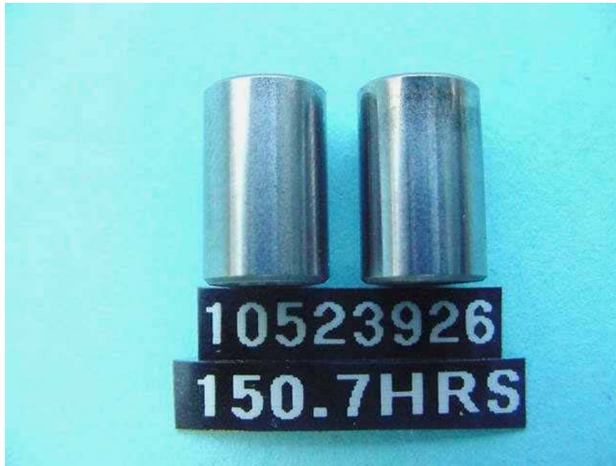
Figure I-1A-10. Test 1 Pump 2: Plunger Assembly Wear
