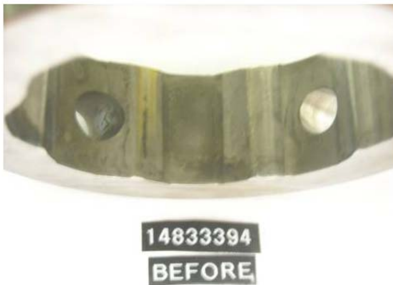
Figure 31 - Pump SN: 14833394 Cam Ring before Testing with R8 + 22.5-ppm DCI-4A Fuel
