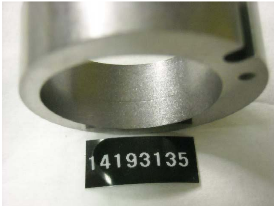
Figure I-1-26. Injection Pump SN:14193135 Transfer Pump Liner Pre-Test Condition
