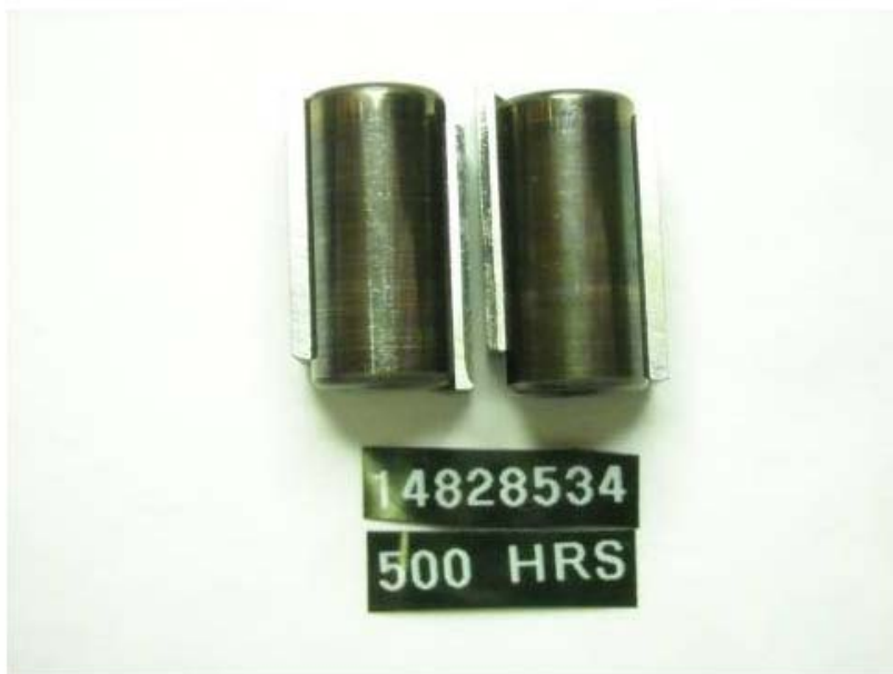
Figure 44 - Pump SN: 14828534 Rollers and Shoe with 500-Hours Testing with R8/JET-A + 22.5-ppm DCI-4A Fuel
