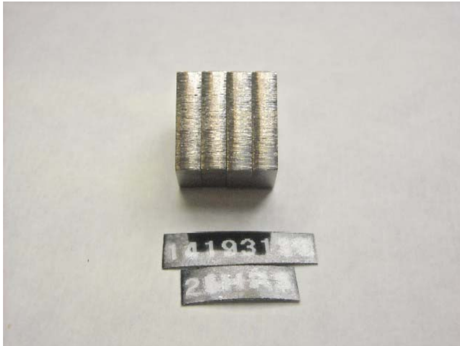
Figure I-1-28. Injection Pump SN:14193135 Transfer Pump Blade Edge Wear
