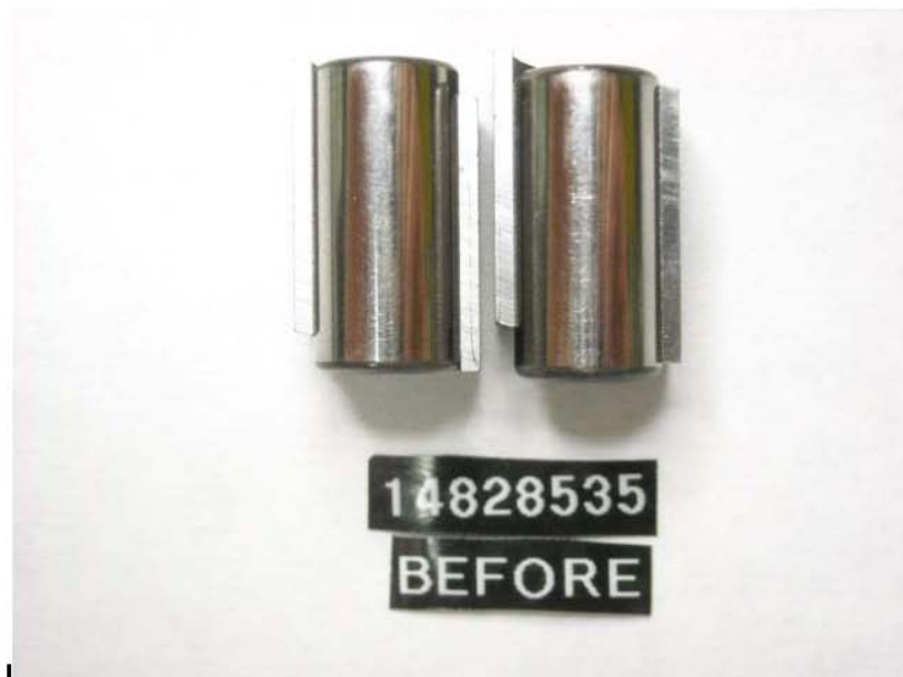
Figure 59 - Pump SN: 14828535 Rollers and Shoe before Testing with R8/JET-A + 22.5-ppm DCI-4A Fuel
