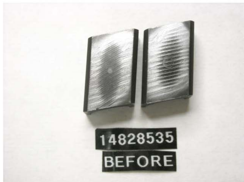
Figure 61 - Pump SN: 14828535 Roller Shoe before Testing with R8/JET-A + 22.5-ppm DCI-4A Fuel
