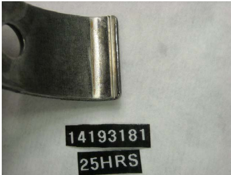
Figure I-1-39. Injection Pump SN:14193181 Leaf Spring/Roller Shoe Wear Contact
