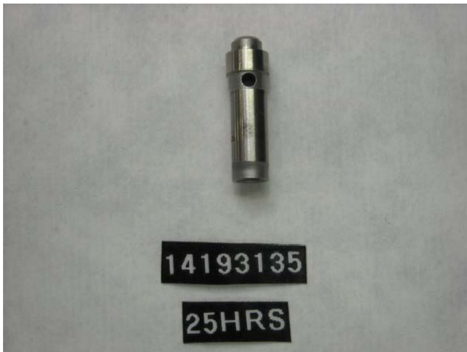
Figure I-1-15. Injection Pump SN:141931335 Delivery Valve Wear Scar
