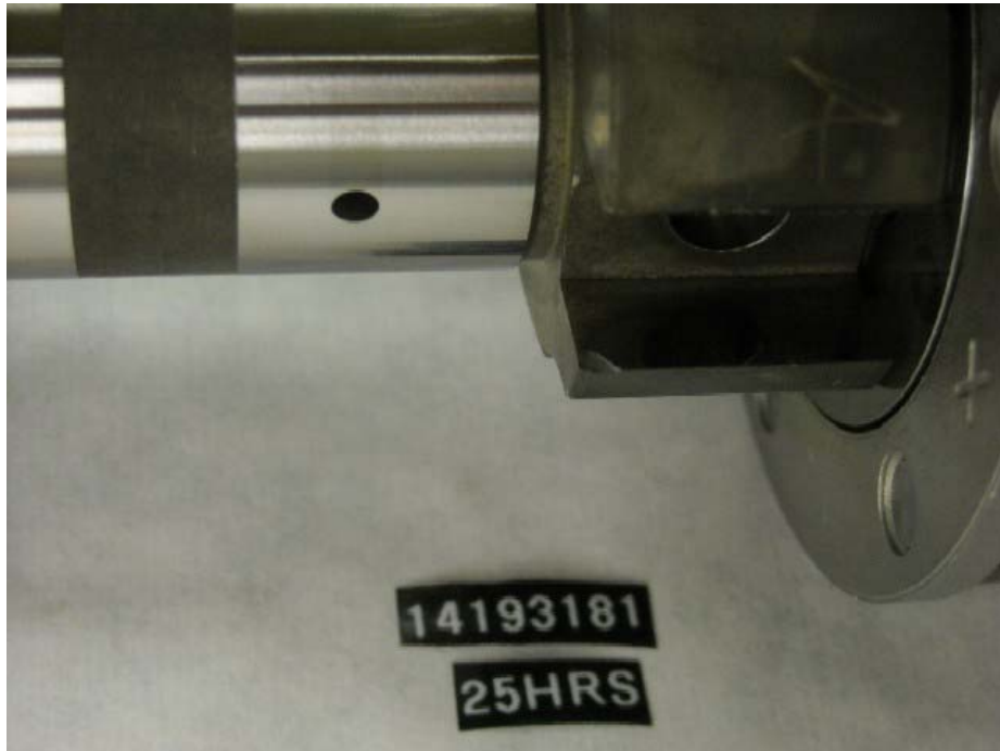
Figure I-1-35. Injection Pump SN:14193181 Drive Shaft with Unusual Chipping in Shoe Slot
