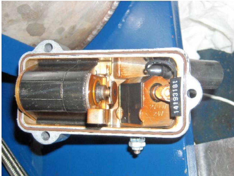
Figure I-1-10. Injection Pump SN:14193181 Top Cover with Deposition and Wear Debris
