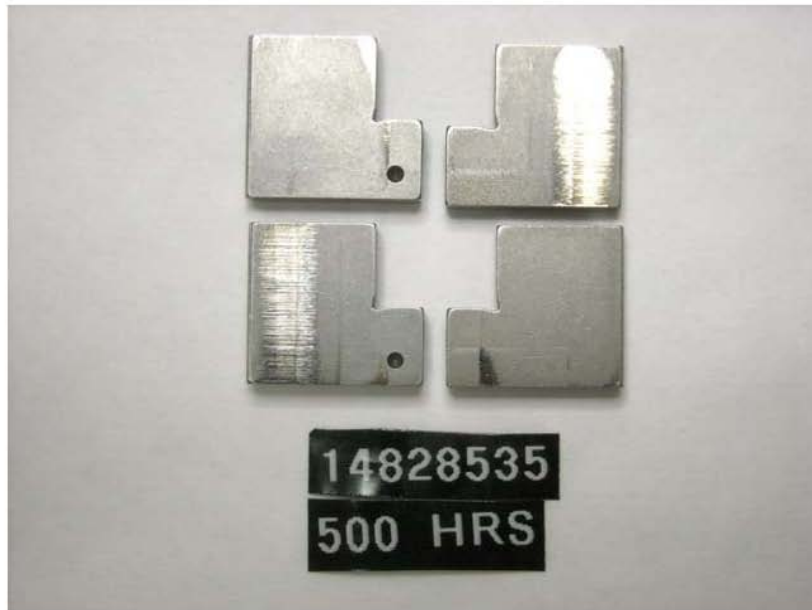
Figure 72 - Pump SN: 14828535 Transfer Pump Blade Sides with 500-Hours Testing with R8/JET-A + 22.5-ppm DCI-4A Fuel
