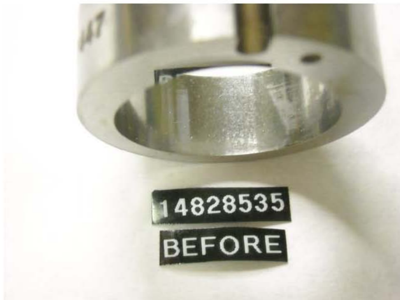
Figure 67 - Pump SN: 14828535 Transfer Pump Liner before Testing with R8/JET-A + 22.5-ppm DCI-4A Fuel
