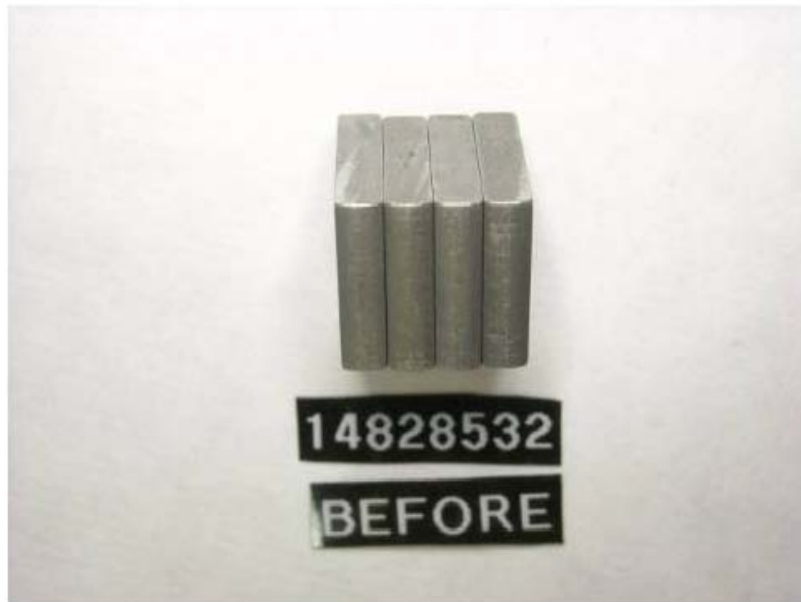
Figure 21 - Pump SN: 14828532 Transfer Pump Blade Edges before Testing with R8 + 22.5-ppm DCI-4A Fuel
