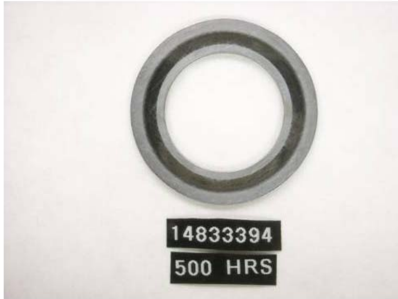
Figure 34 - Pump SN: 14833394 Thrust Washer with 500-Hours Testing with R8 + 22.5-ppm DCI-4A Fuel
