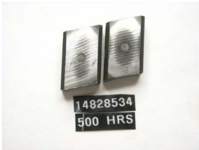
Figure 46 - Pump SN: 14828534 Roller Shoe with 500-Hours Testing with R8/JET-A + 22.5-ppm DCI-4A Fuel
