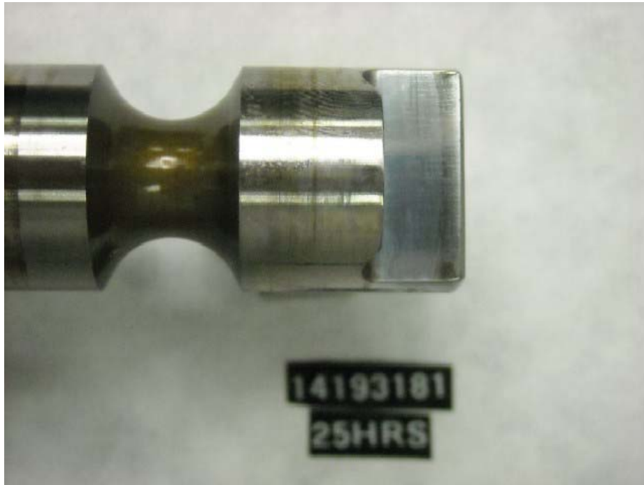
Figure I-1-33. Injection Pump SN:14193181 Rotor Drive Tang with Minimal Wear
