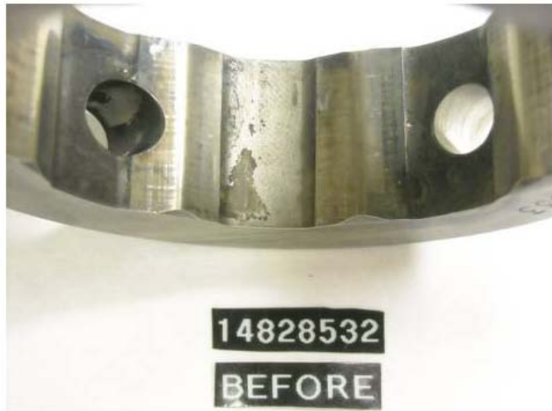
Figure 15 - Pump SN: 14828532 Cam Ring before Testing with R8 + 22.5-ppm DCI-4A Fuel
