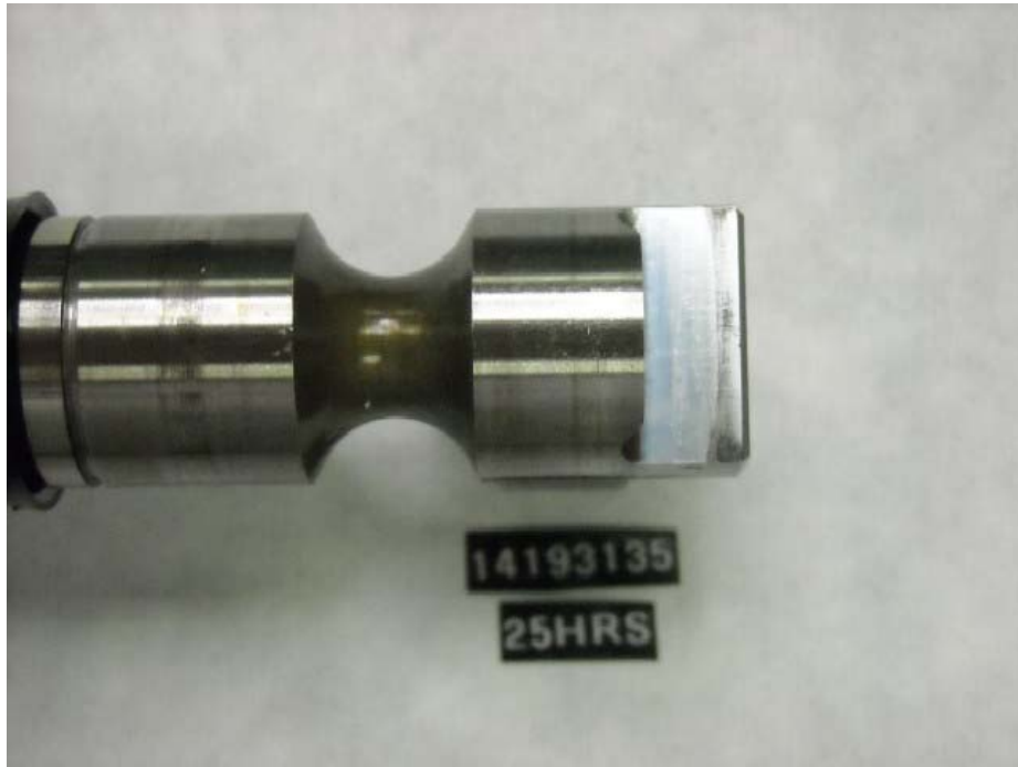
Figure I-1-12. Injection Pump SN:14193135 Rotor Drive Tang with Minimal Wear
