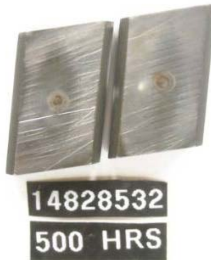
Figure 14 - Pump SN: 14828532 Roller Shoe with 500-Hours Testing with R8 + 22.5-ppm DCI-4A Fuel
