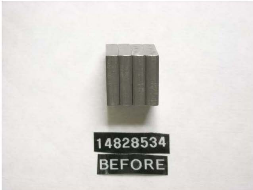
Figure 53 - Pump SN: 14828534 Transfer Pump Blade Edges before Testing with R8/JET-A + 22.5-ppm DCI-4A Fuel
