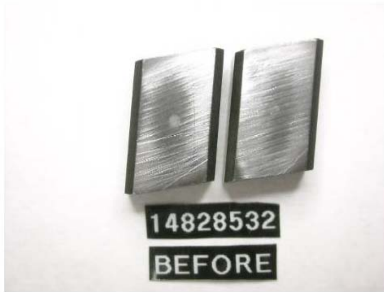
Figure 13 - Pump SN: 14828532 Roller Shoe before Testing with R8 + 22.5-ppm DCI-4A Fuel
