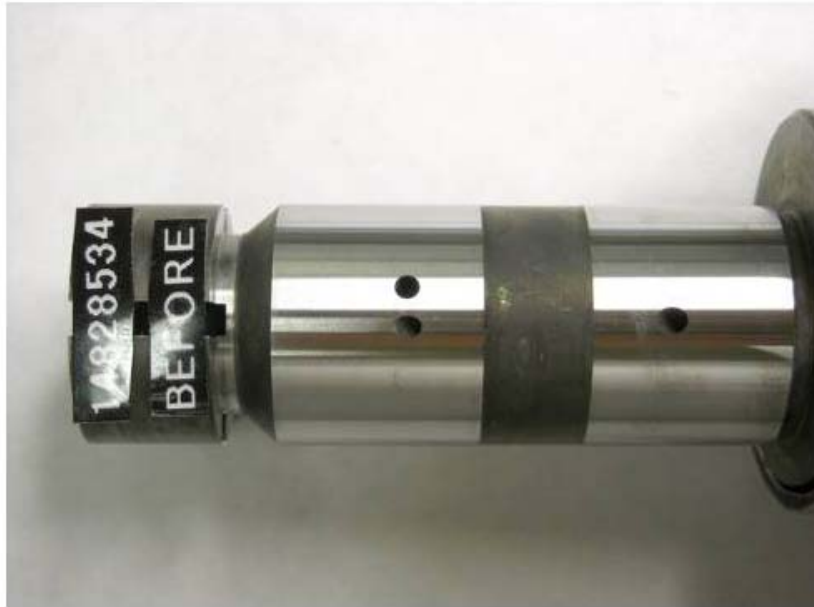
Figure 41 - Pump SN: 14828534 Distributor Rotor before Testing with R8/JET-A + 22.5-ppm DCI-4A Fuel
