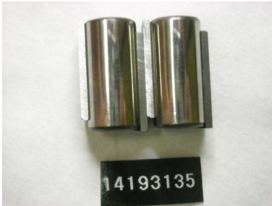
Figure I-1-16. Injection Pump SN:14193135 Pre-Test Roller Shoes and Rollers
