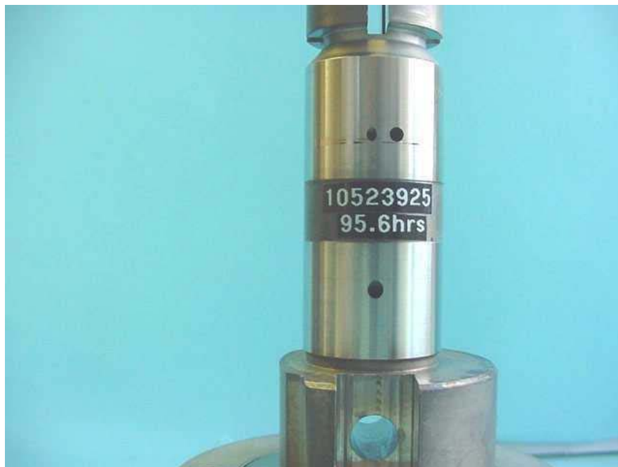
Figure I-1A-11. Test 1 Pump 1: Rotor Shaft Wear
