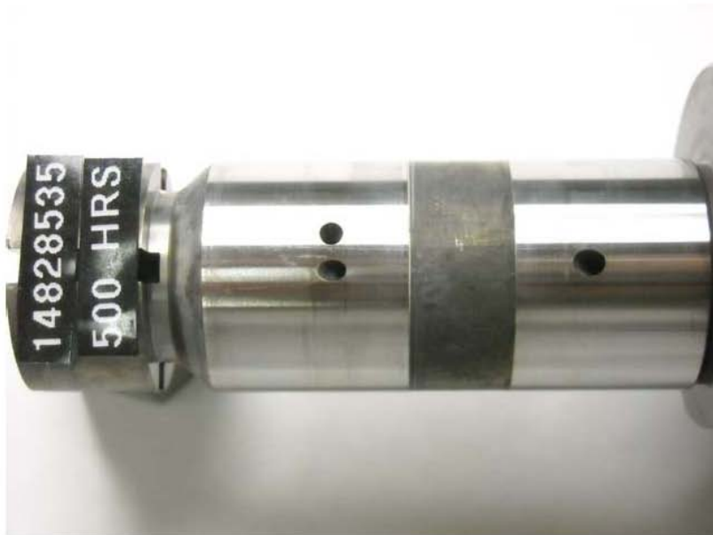
Figure 58 - Pump SN: 14828535 Distributor Rotor with 500-Hours Testing with R8/JET-A + 22.5-ppm DCI-4A Fuel
