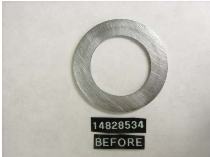
Figure 49 - Pump SN: 14828534 Thrust Washer before Testing with R8/JET-A + 22.5-ppm DCI-4A Fuel
