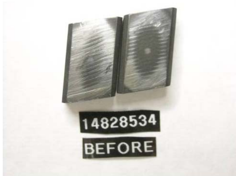
Figure 45 - Pump SN: 14828534 Roller Shoe before Testing with R8/JET-A + 22.5-ppm DCI-4A Fuel
