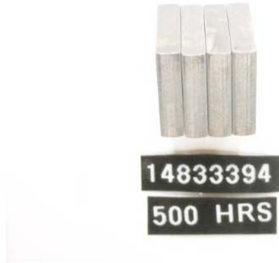
Figure 38 - Pump SN: 14833394 Transfer Pump Blade Edges with 500-Hours Testing with R8 + 22.5-ppm DCI-4A Fuel
