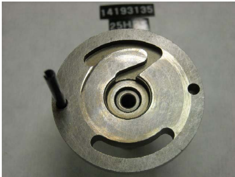
Figure I-1-31. Injection Pump SN:14193135 Transfer Pump Regulator Wear
