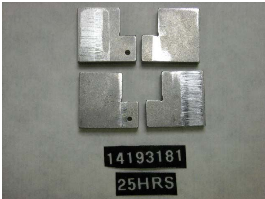
Figure I-1-50. Injection Pump SN:14193181 Transfer Pump Blade Side Wear
