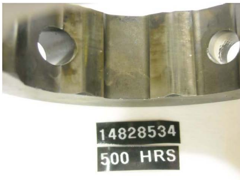
Figure 48 - Pump SN: 14828534 Cam Ring with 500-Hours Testing with R8/JET-A + 22.5-ppm DCI-4A Fuel
