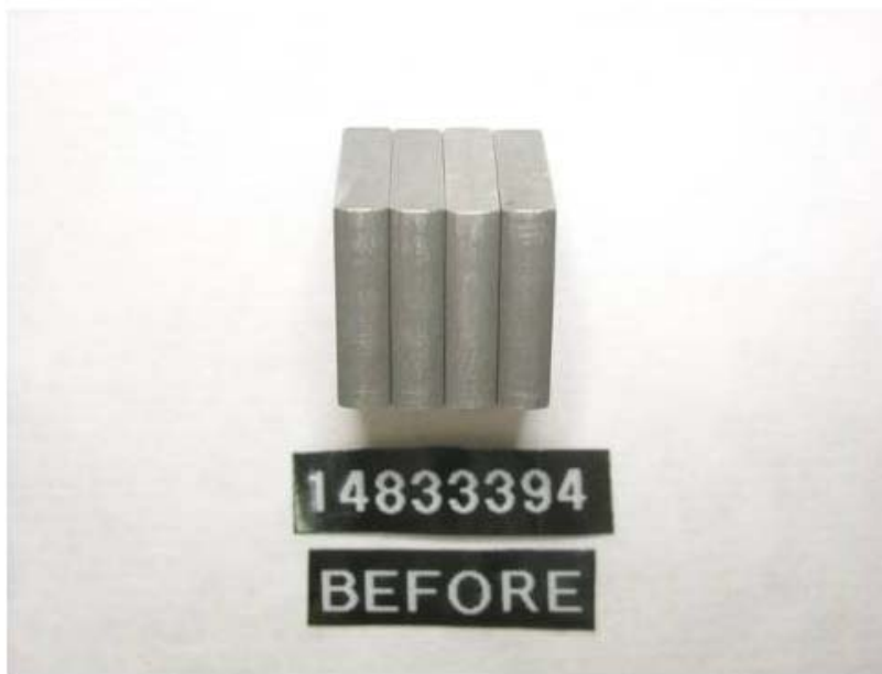
Figure 37 - Pump SN: 14833394 Transfer Pump Blade Edges before Testing with R8 + 22.5-ppm DCI-4A Fuel
