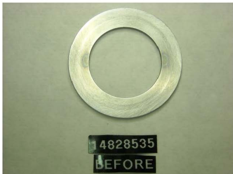
Figure 65 - Pump SN: 14828535 Thrust Washer before Testing with R8/JET-A + 22.5-ppm DCI-4A Fuel
