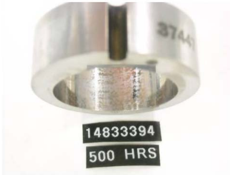
Figure 36 - Pump SN: 14833394 Transfer Pump Liner with 500-Hours Testing with R8 + 22.5-ppm DCI-4A Fuel
