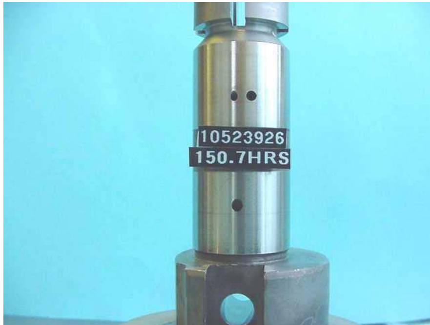
Figure I-1A-12. Test 1 Pump 2: Rotor Shaft Wear
