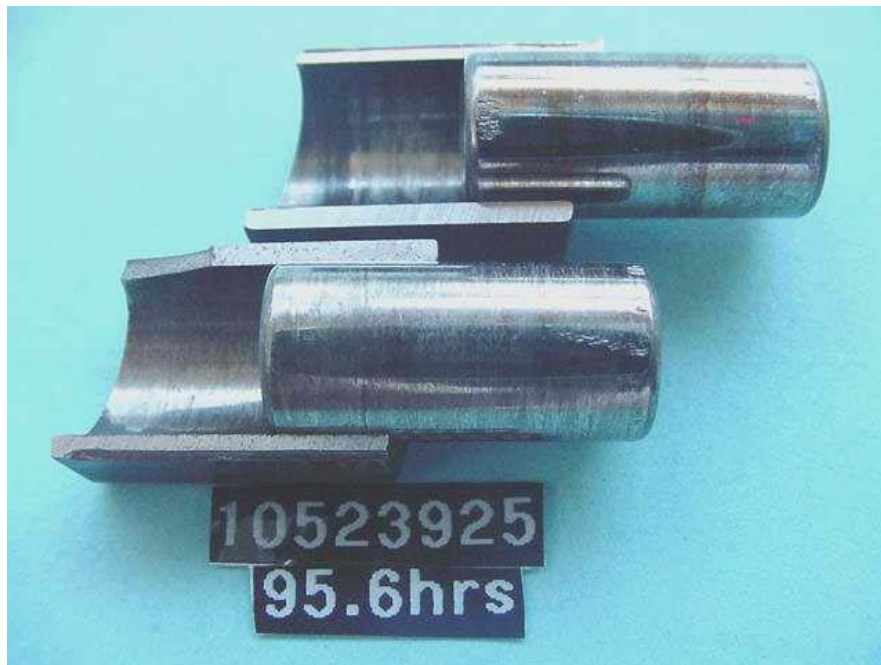
Figure I-1A-5. Test 1 Pump 1: Chipped Shoe Wear
