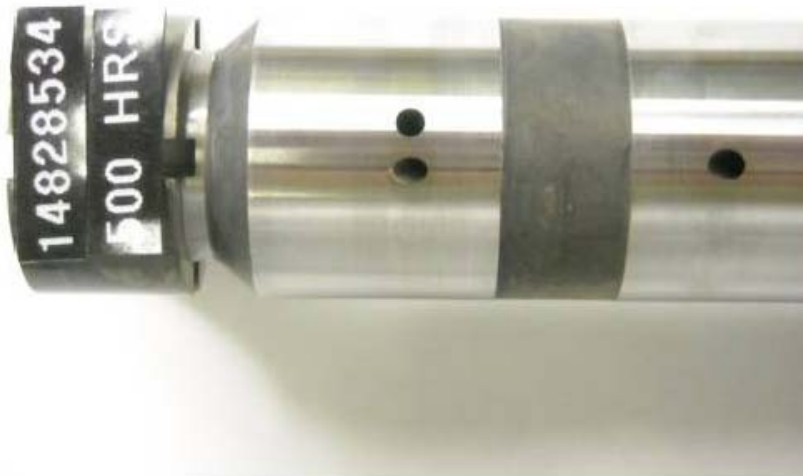
Figure 42 - Pump SN: 14828534 Distributor Rotor with 500-Hours Testing with R8/JET-A + 22.5-ppm DCI-4A Fuel
