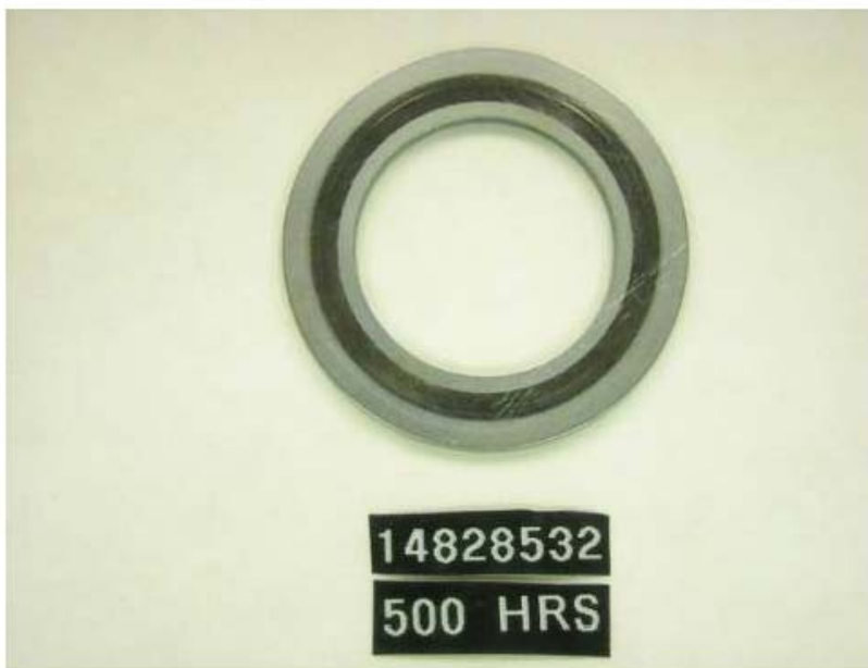
Figure 18 - Pump SN: 14828532 Thrust Washer with 500-Hours Testing with R8 + 22.5-ppm DCI-4A Fuel
