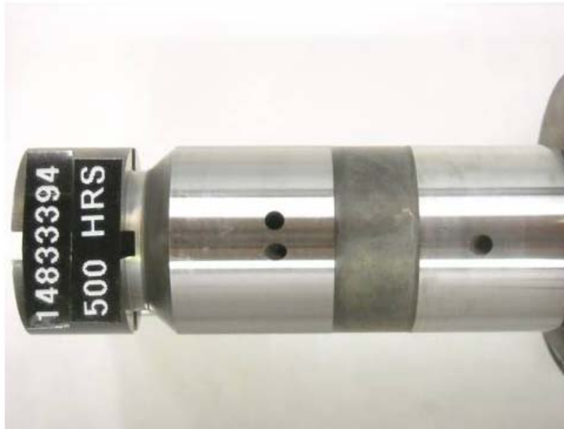
Figure 26 - Pump SN: 14833394 Distributor Rotor with 500-Hours Testing with R8 + 22.5-ppm DCI-4A Fuel
