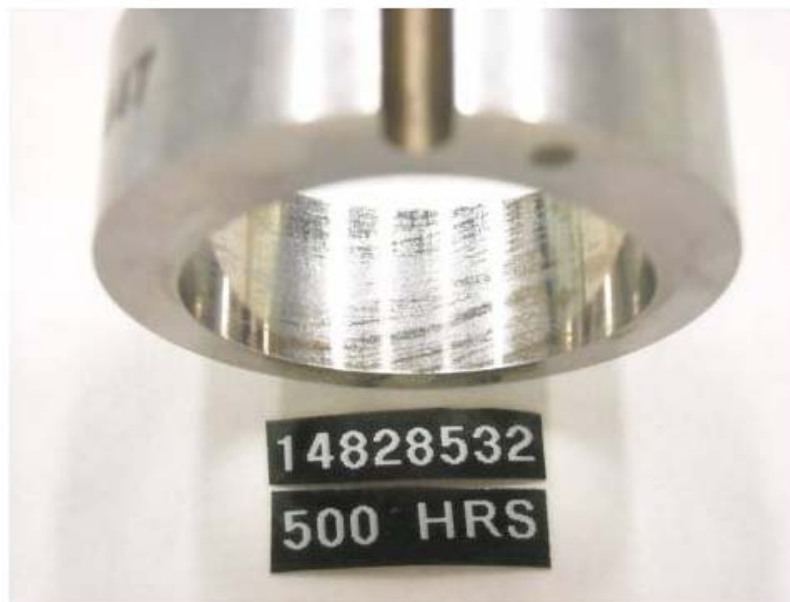
Figure 20 - Pump SN: 14828532 Transfer Pump Liner with 500-Hours Testing with R8 + 22.5-ppm DCI-4A Fuel
