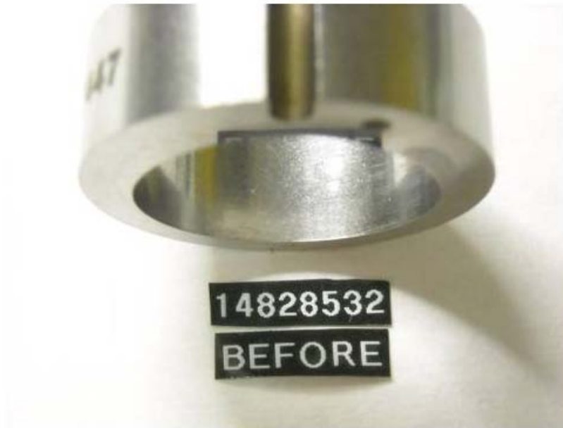
Figure 19 - Pump SN: 14828532 Transfer Pump Liner before Testing with R8 + 22.5-ppm DCI-4A Fuel
