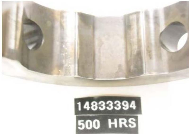
Figure 32 - Pump SN: 14833394 Cam Ring with 500-Hours Testing with R8 + 22.5-ppm DCI-4A Fuel
