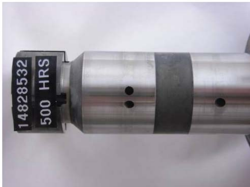
Figure 10 - Pump SN: 14828532 Distributor Rotor with 500-Hours Testing with R8 + 22.5-ppm DCI-4A Fuel
