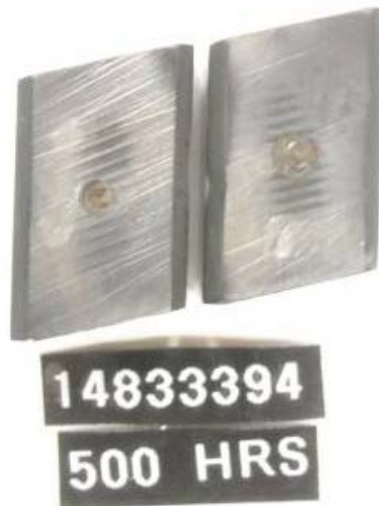
Figure 30 - Pump SN: 14833394 Roller Shoe with 500-Hours Testing with R8 + 22.5-ppm DCI-4A Fuel
