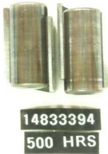
Figure 28 - Pump SN: 14833394 Rollers and Shoe with 500-Hours Testing with R8 + 22.5-ppm DCI-4A Fuel
