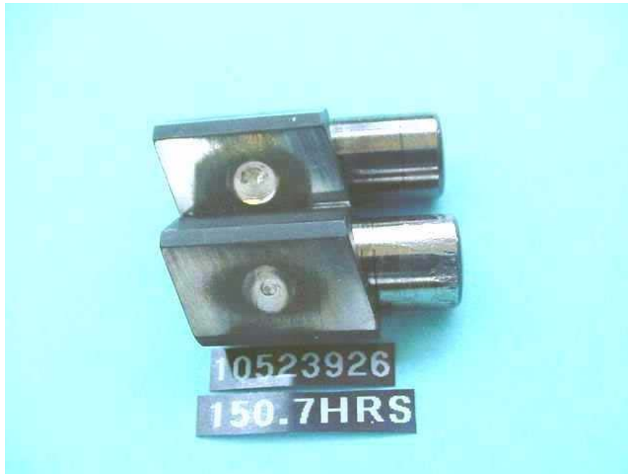
Figure I-1A-8. Test 1 Pump 2: Shoe Back and Roller Wear
