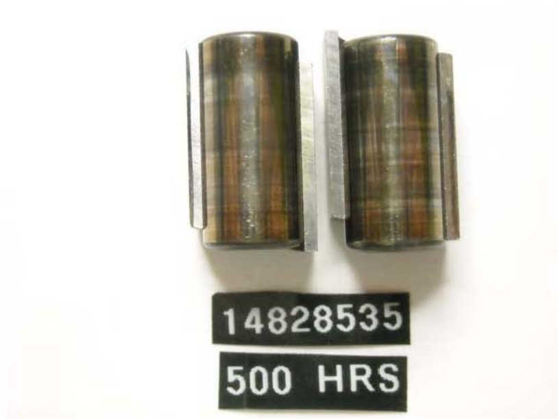
Figure 60 - Pump SN: 14828535 Rollers and Shoe with 500-Hours Testing with R8/JET-A + 22.5-ppm DCI-4A Fuel
