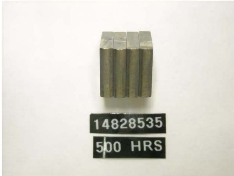
Figure 70 - Pump SN: 14828535 Transfer Pump Blade Edges with 500-Hours Testing with R8/JET-A + 22.5-ppm DCI-4A Fuel
