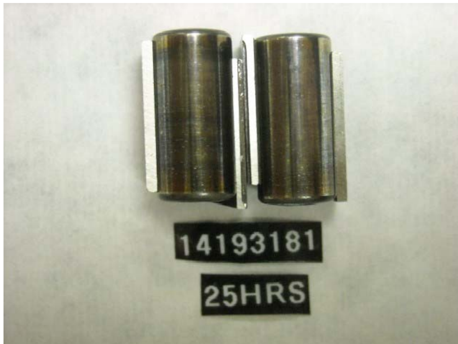
Figure I-1-38. Injection Pump SN:14193181 25-Hour R-8 Fuel Roller Shoes and Rollers
