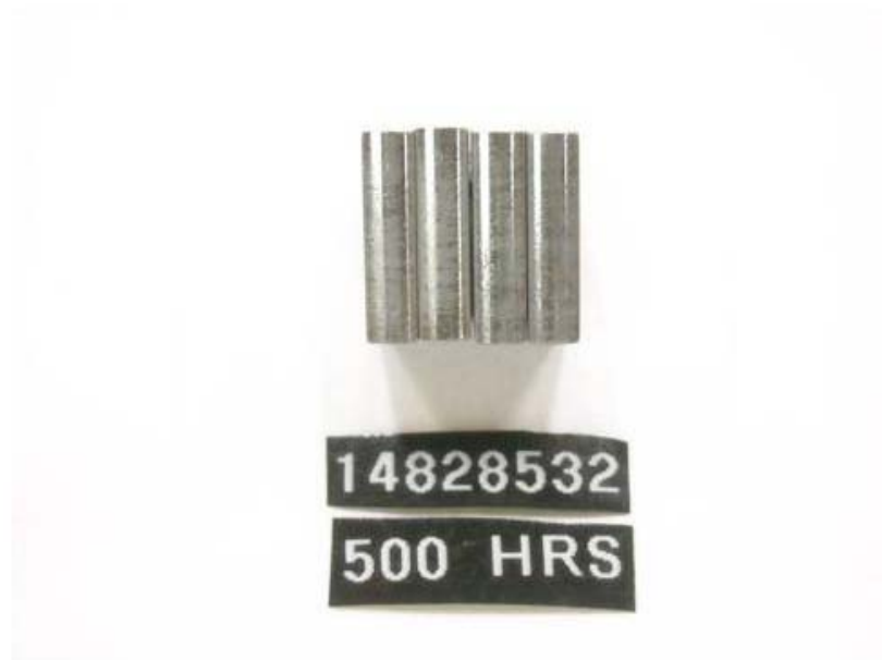
Figure 22 - Pump SN: 14828532 Transfer Pump Blade Edges with 500-Hours Testing with R8 + 22.5-ppm DCI-4A Fuel
