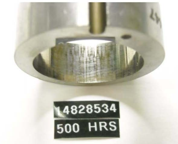
Figure 52 - Pump SN: 14828534 Transfer Pump Liner with 500-Hours Testing with R8/JET-A + 22.5-ppm DCI-4A Fuel
