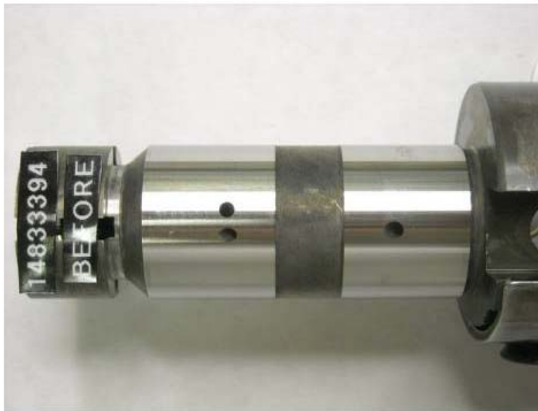
Figure 25 - Pump SN: 14833394 Distributor Rotor before Testing with R8 + 22.5-ppm DCI4A Fuel
