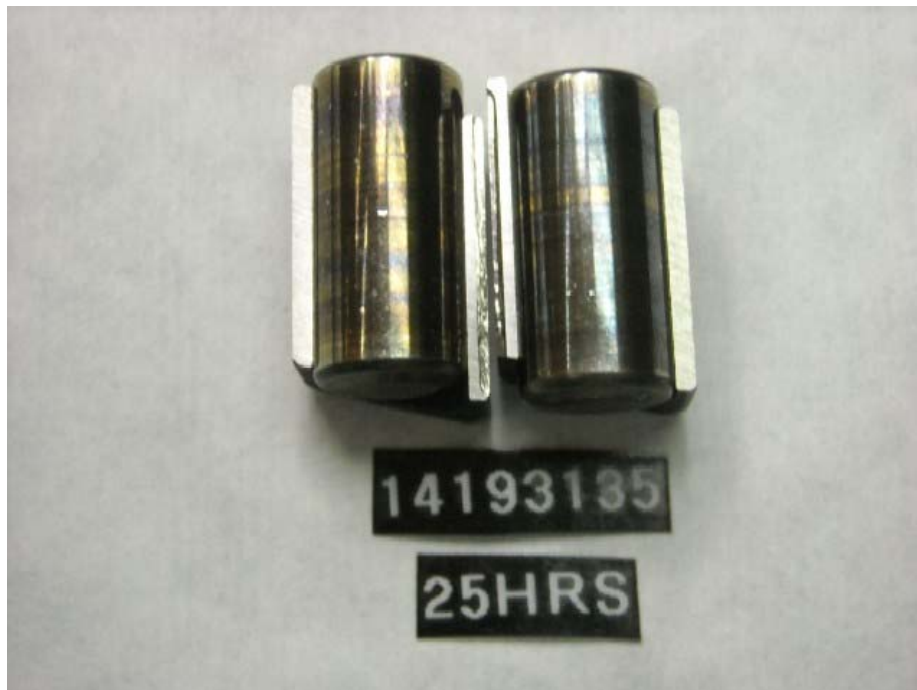
Figure I-1-17. Injection Pump SN:14193135 25-Hour R-8 Fuel Roller Shoes and Rollers
