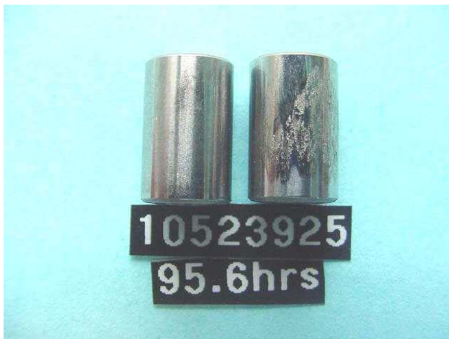
Figure I-1A-9. Test 1 Pump 1: Plunger Assembly Wear
