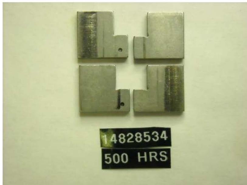
Figure 56 - Pump SN: 14828534 Transfer Pump Blade Sides with 500-Hours Testing with R8/JET-A + 22.5-ppm DCI-4A Fuel
