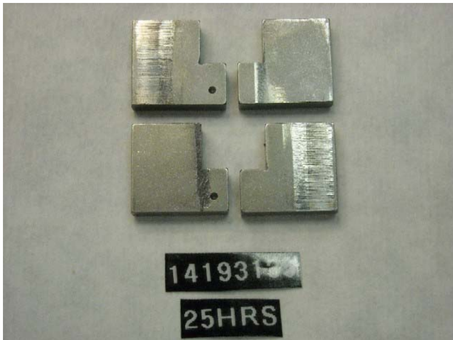
Figure I-1-29. Injection Pump SN:14193135 Transfer Pump Blade Side Wear
