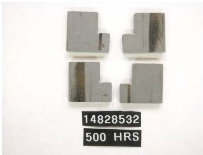
Figure 24 - Pump SN: 14828532 Transfer Pump Blade Sides with 500-Hours Testing with R8 + 22.5-ppm DCI-4A Fuel
