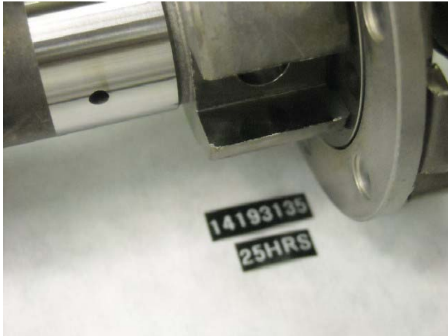
Figure I-1-14. Injection Pump SN:141931335 Drive Shaft with Unusual Chipping in Shoe Slot
