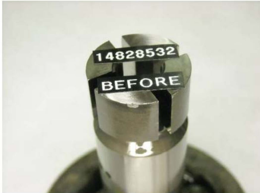
Figure 8 - Pump SN: 14828532 Distributor Rotor Transfer Pump Blade Slots with Chip before Testing with R8 + 22.5-ppm DCI-4A Fuel
