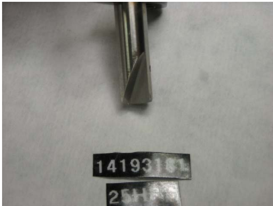
Figure I-1-46. Injection Pump SN:14193181 Metering Valve Wear
