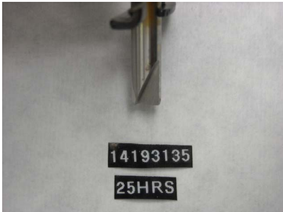
Figure I-1-25. Injection Pump SN:14193135 Metering Valve Wear
