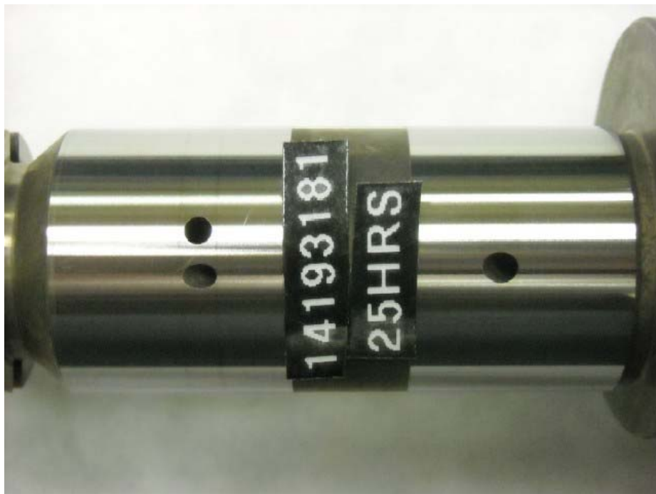
Figure I-1-34. Injection Pump SN:14193181 Rotor Discharge Ports with Minimal Wear
