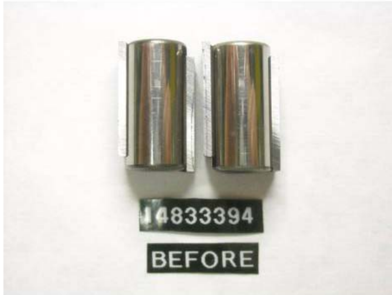
Figure 27 - Pump SN: 14833394 Rollers and Shoe Condition before Testing with R8 + 22.5-ppm DCI-4A Fuel
