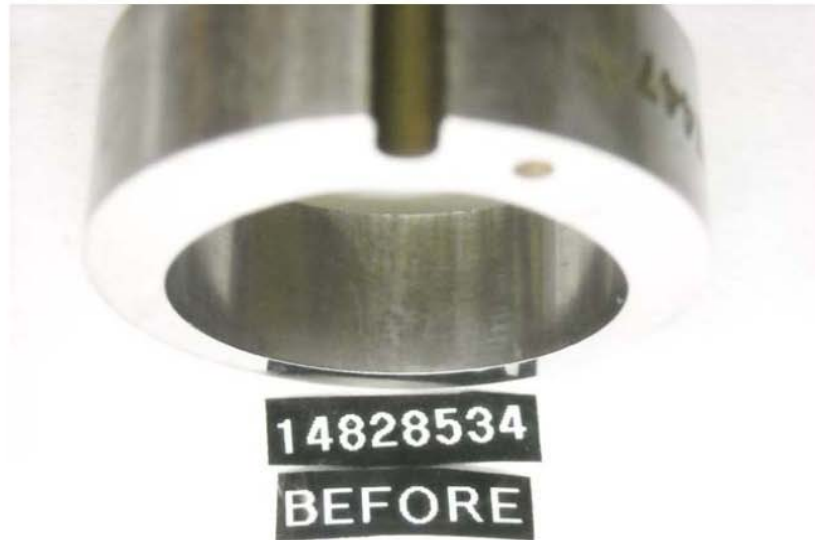
Figure 51 - Pump SN: 14828534 Transfer Pump Liner before Testing with R8/JET-A + 22.5-ppm DCI-4A Fuel
