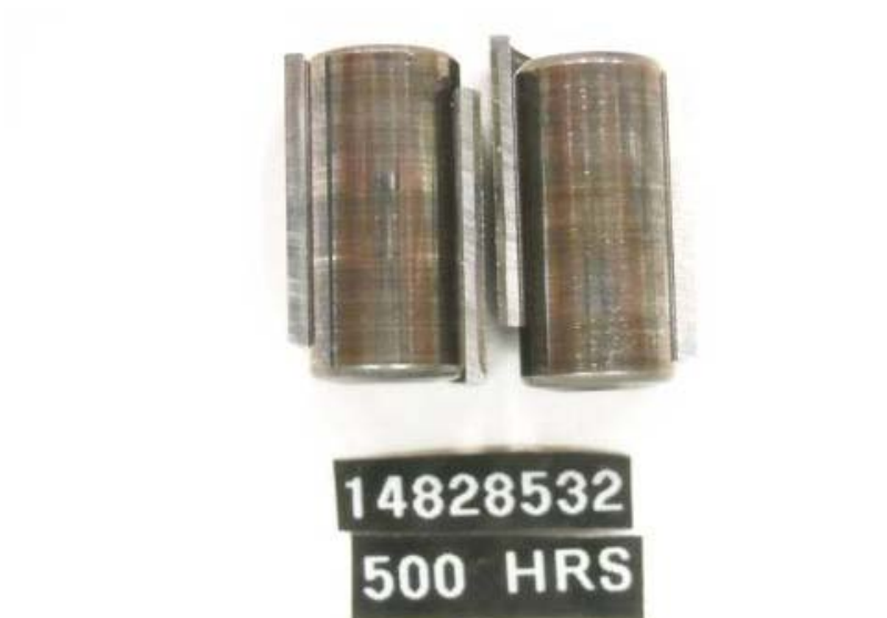
Figure 12 - Pump SN: 14828532 Rollers and Shoe with 500-Hours Testing with R8 + 22.5-ppm DCI-4A Fuel
