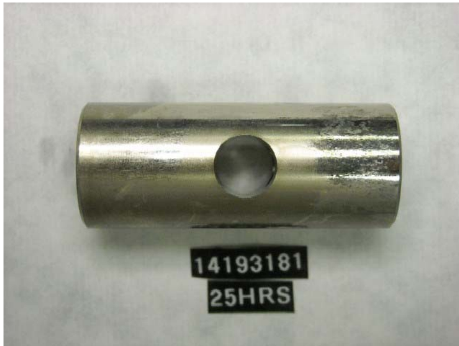
Figure I-1-45. Injection Pump SN:14193181 Advance Piston Wear
