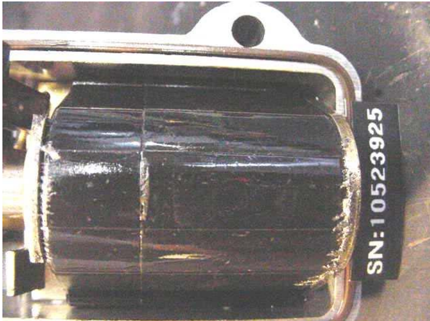
Figure I-1A-2. Test 1 Pump 1: Metal Shavings on Solenoid
