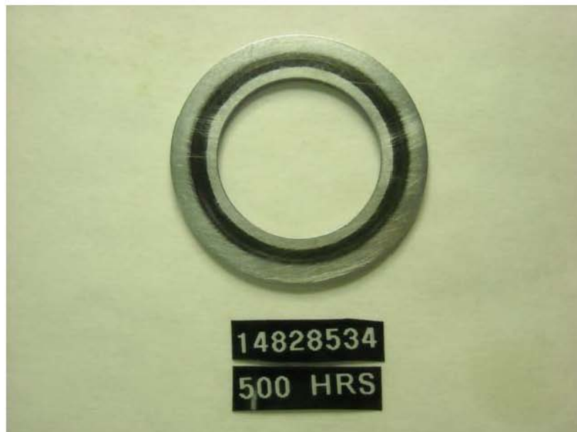
Figure 50 - Pump SN: 14828534 Thrust Washer with 500-Hours Testing with R8/JET-A + 22.5-ppm DCI-4A Fuel
