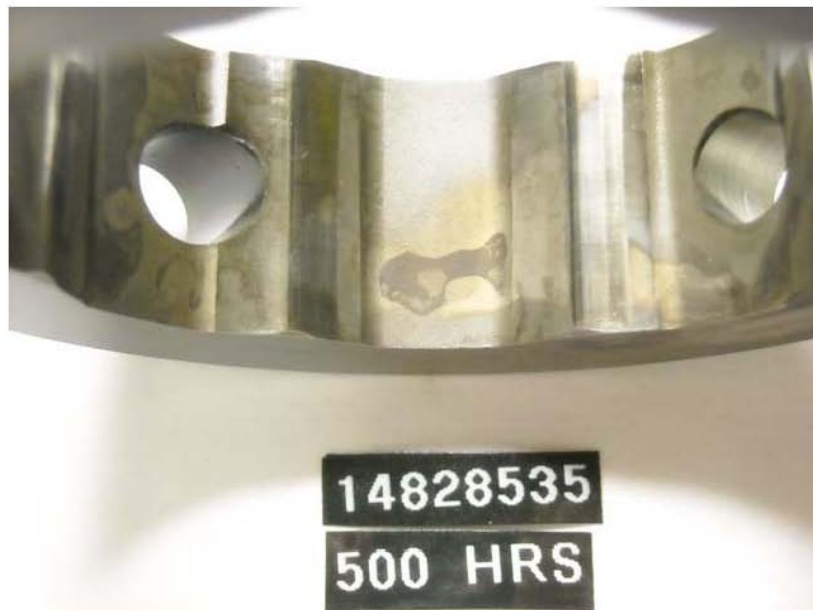
Figure 64 - Pump SN: 14828535 Cam Ring with 500-Hours Testing with R8/JET-A + 22.5-ppm DCI-4A Fuel
