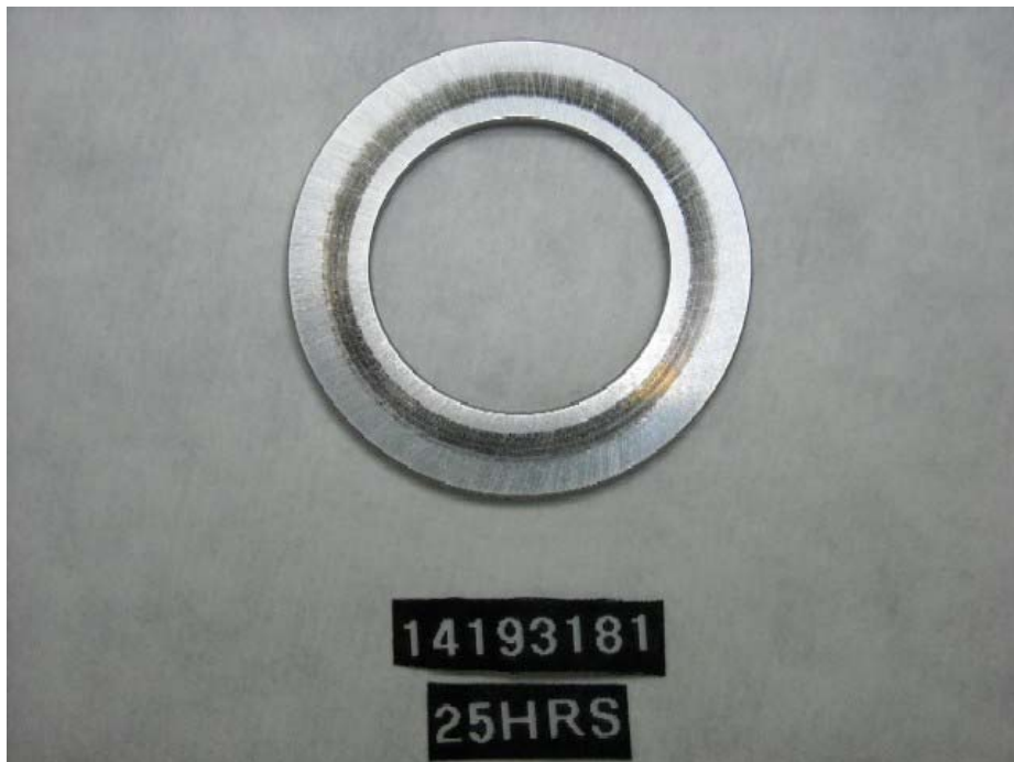
Figure I-1-44. Injection Pump SN:14193181 Governor Weight Thrust Washer
